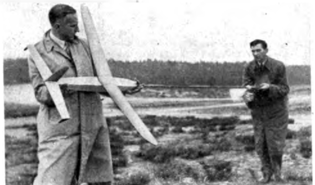
Below: The Belgian corner with Deschepper and pipe, in centre. Diamond fuselages, with unusual built-up 'spine' wing mounting platforms were features of the Belgian models. Deschepper used a variable pitch prop on his entry.
