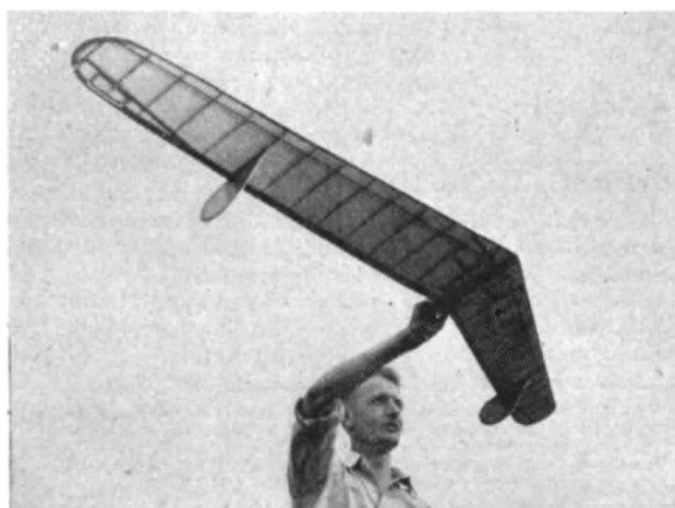
Roy Yeabsley is currently flying a 7-ft. tailless sailplane in rallies and contests. Seen here at the Northern Heights Gata, the lightweight structure, moderate sweepback and usual underslung fins are points to note.
