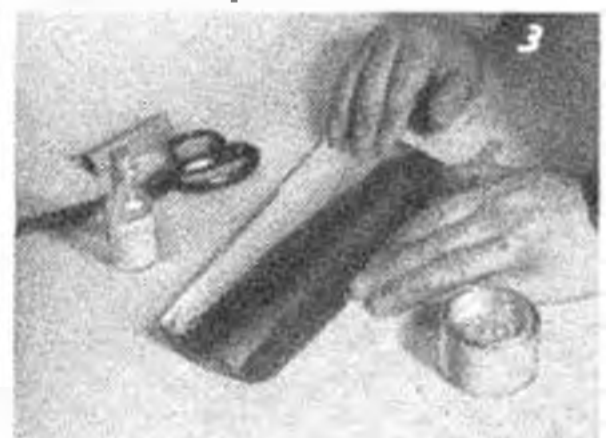
1. Etching the gluing area with sandpaper, shears or scissors cut the metal easily. 2. Gluing the balsa with special adhesive; note reflection from highly polished surface. 3. Folded over the framework and held for 10 minutes, the result is a perfect wing for control line speed.
