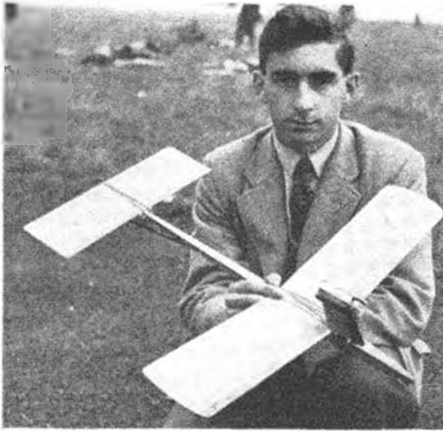
Dick Tironey, who favors a high thrustline, has pylon mounted motor and slender underfin on his '52 entry for the I.C.I. Challenge Trophy. Span is only 24 inches.
