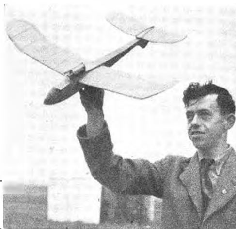
K. D. Mole of Tynemouth and his version of Dick Ticeoney's Ticeizer design, available through A.P.S. An easy model to build and trim. Jetex 200 unit is used; span is 26 inches.
