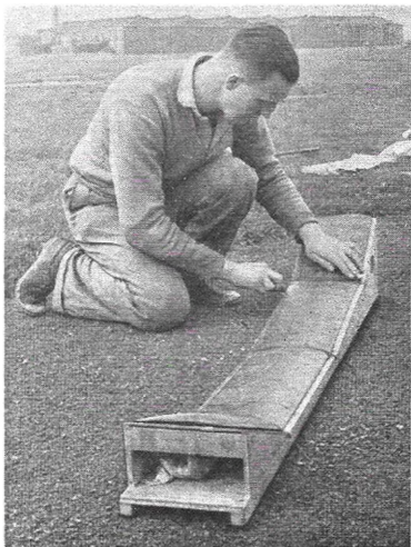
Jim Waldron straps down by means of wide rubber bands, the wings of his International Class power model. Henley Club anti-warp boards are a regular feature at S.M. Area meetings, and have certainly paid the Club dividends over the past few seasons
