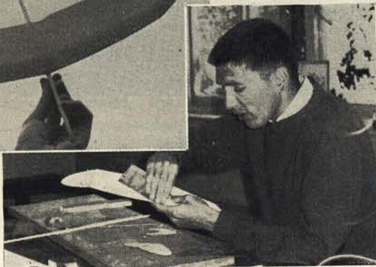
Just evident in the plan view of "Sweepette" is the sharp ridge line at the maximum airfoil camber point. Lee at work in the editorial offices, uses the sandpaper block to finish his well constructed wing.
