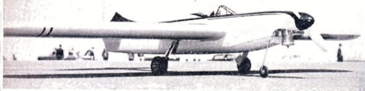
Left, Sandy Pinkert with Don Pinkert's 173 m.p.h. S.T. .29RV speed model, Florida. 60 per cent Nitro, 20 per cent Castor Oil, 5 per cent N. Benzine, 15 per cent Methanol. Below left, S.T. 40RV powered "Hoptee" by Art Adamisin, Detroit. Note long tank with Quick Fill Valve. Below, John Kilsdonk, "Hoptee" designer M.A.N. plan 67A.
