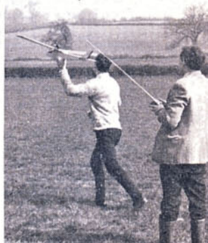
Field procedure with "Apprentice", a simple pylon mounted engine powered model. Left, start the engine with an assistant holding the model and positioning the glow plug leads onto the engine. Right, check the radio for the last time with the engine running, launch from shoulder height.
