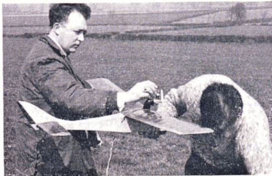
Field procedure with "Apprentice", a simple pylon mounted engine powered model. Left, start the engine with an assistant holding the model and positioning the glow plug leads onto the engine. Right, check the radio for the last time with the engine running, launch from shoulder height.
