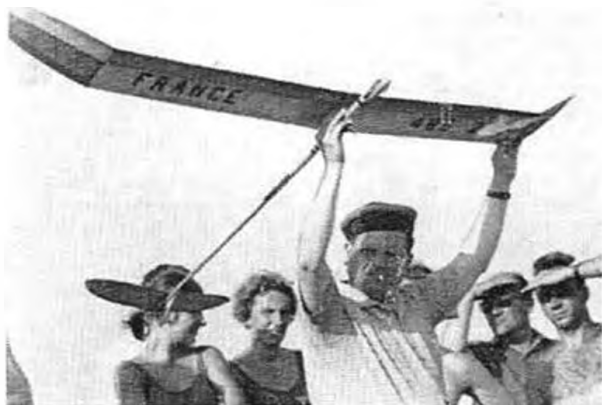
Jean-Marie Berthe's A/2 which made the longest flight in the fly-off but didn't win, was beautifully built; it featured a flamingo airfoil, pylon mounted wing and an offset towhook to counteract the permanently set glide turn.
