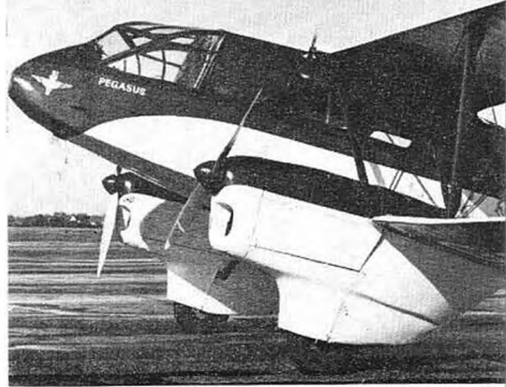
Views on this page, show details of Pegasus, the Rothman Rapide used for the Airborne Regt. to practice skydiving and photographed for us by C. S. West at Blackbushe. Above: the shape of the nose, cabin external detail and the engine nacelle are helpful for modellers. Left, and Below, are more details of the nacelle and main undercarriage. Note from these pictures that the nacelles are not handed but identical, i.e. exhaust pipes and intakes on the starboard side whilst cooling openings are to port. The nacelles are only the intricate part of a D.H. 89A for model reproduction and present a problem through the sharp taper at the rear under the wing exactly where the engine bearers have to be mounted! (See sketch opposite.) Note also the cabin window frames, doubled drag and landing wires in inner bay and strut positions.
