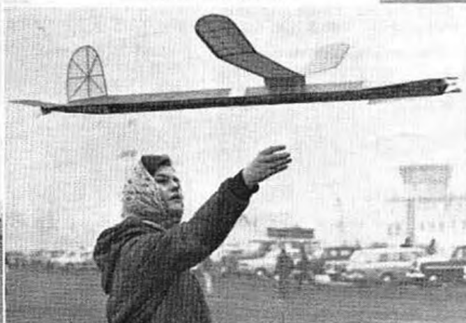
Top left: Peterborough's M. Page had a 12 x 120 ins. plank in tailless weighing 32 oz. and with the Swiss S-1 airfoil. Winner of the event Ken Attwell flew rubber tailless with a pop-up 44 in. wing and rearward folding 23 x 26 ins. prop as in next photo. Top right is Doug McHard, releasing delightful Bristol Fighter indoor rubber scale to amazement of Comp. Secy. G. Lynn (check shirt) and other nonchalant onlooker. At left: Women's Cup winner Mary Day shows the way to launch, so too does Jennifer Edwards, test gliding (below) and Sue Miller with Climax power design at right. These ladies filled first three places in their event, Sue also placed second in the Open Power contest.
