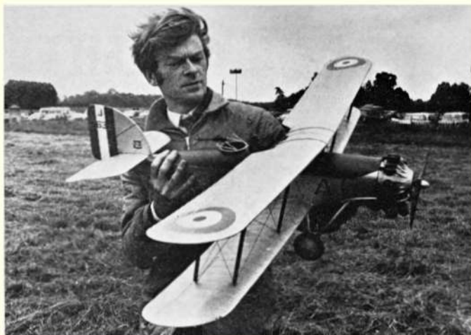
Vic Driscoll of St. Albans flew this magnificent free flight Westland Wapiti so impressively it became clear winner of its class at our Annual All-Scale Rally this year at Old Warden. It weighs 30oz., uses a Marown Snipe 1.5 c.c. diesel.
