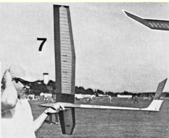
1. Chmelik (Austria) uses wing sheet covered top and bottom. 2. Elton Drew's new still-air A/2—note turbulator forward of L.E. 3. Two-piece fuselage—hardwood front, balsa tube rear, used by Cosma. Eggbox construction rear of sheeted L.E. 4. Australian model of Pete Nitschke in the hands of Jan Zetterfall and sister Ann. 5. Dave Linstrum (hatted) and Tom Hutchinson with Dennis Bronco's elegant machine. 6. Ex-Wakefield winner Löffler with Hirschel's A/2. 7. Tee-tail, straight dihedral wing used by Nummukka. 8. Another view of Nitschke's proxy flown, rather old fashioned looking design. Shirt inscription reads 'Eat more porridge!'. 9. Cuban A/2 of Marsella, held here by Menendez. Nicely finished with contrasting tissue trim. 10. North Korean team member Hong Sun Hen, with colleague using walkie-talkie. 11. Tom Hutchinson (editor of Sun Valeers Newsletter) releases Langerin's A/2.
