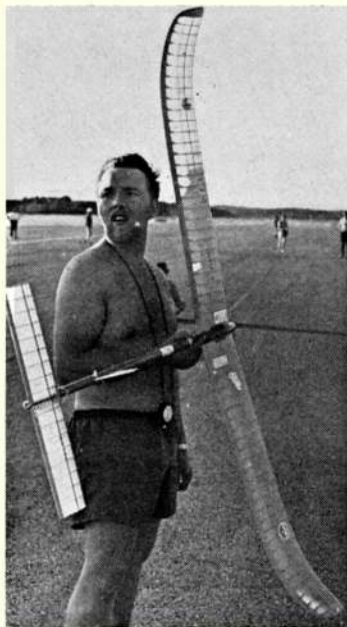
Larsen's A/2 has unusual curved wing dihedral. Note also the fin position - midway down the fuselage. Placed 19th.
