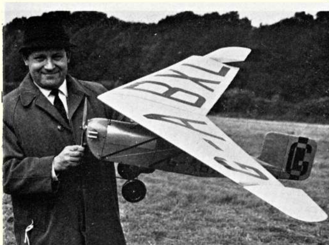
Dennis Bryant produced his remarkable Grainger Archaeopteryx tailless scale R/C model and it was awarded the Shuttleworth Trophy as most outstanding replica of a Museum subject. 75 in. span, it has a Merco 29 and tip controls. Real machine is also flying from Old Warden. Top right is the power department on the Albatros DV by R. Geall to 1/6th scale. Merco 61 is completely hidden, Dummy exhaust valves, water coolant pipes and exhausts look fine in a glass fibre structure fuselage.
