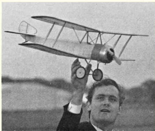
Another advocate of 'painting when proved' is J. Turvey, seen here test gliding his unpainted Sopwith 1 1/2 Strutter, built to 1/12th scale, and powered by a Mills .75 c.c.
