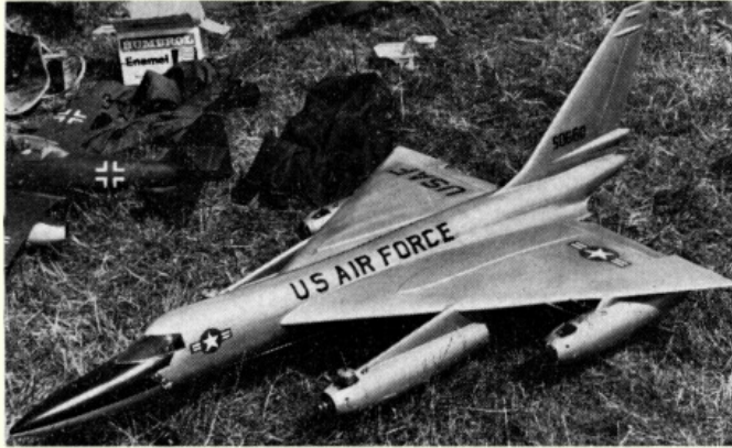
Another Mike Ennis C/L project - a Hustler B58 powered by four PAW 19s (although only two fitted at the moment). Model as yet unflown, but is designed to take-off from a 'dolly' and has reinforced nacelles to take landing shocks. Weighs 5 lb.
