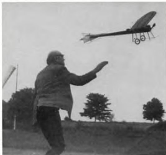
Electric power (a Mabuchi 36D) is used by Alan Palfrey for his 1910 Henriot Monoplane , and it provides a nice, slow and steady flight pattern. Batteries recharge via dry cells.
