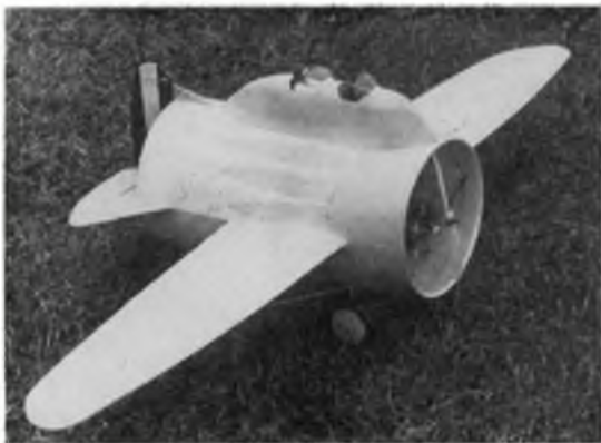
Above: You will not find many more original aircraft than the Stepa Caproni as a modelling subject – this C/L version was built by J. Gudge to 1/12th scale for an Enya 19. Yes, it does fly – even looped! At right is nice engine detail on Mike Ennis' Pfalz D3 control liner, built to 1/4th scale.
