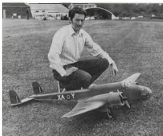
Winner of the prize for best C/L model was Ron Truelove once again with bomb dropping Handley Page Hampden. Undercarriage retracts and flaps operate on this huge, most impressive model. Outer wing tip panels detach to ease transport problems. Uses a pair of throttle equipped OS40 engines for power.
