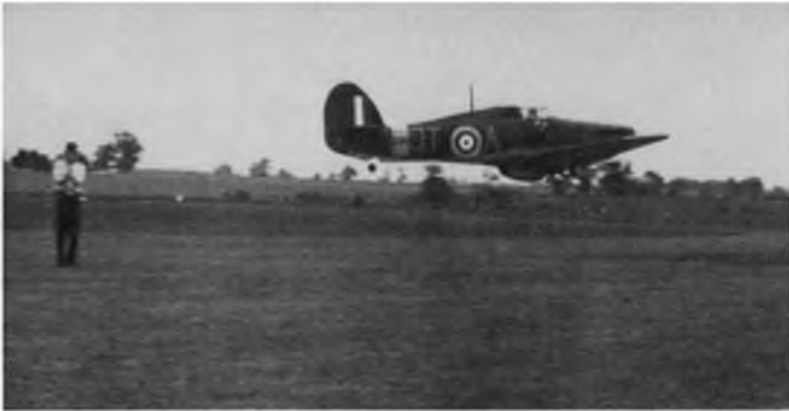
Vic Willson flies his Mick Reeves kitted Hurricane with both radio control as well as control line, making it a very useful dual purpose model. Using his familiar closed-loop R/C type control line handle, he had perfect control over the throttle in this huge (80in. span) model – but centrifugal force prevented one of the undercarriage legs from retracting properly. No problems though when it flies purely R/C. At right is Three Kings member Ken Gardner with his C/L Tomtit which won the Jack Carter Memorial Trophy for best C/L bipe. Built from the Veron R/C kit and powered by an OS58, it weighs 7lbs. 2oz. and uses Solarfilm covering.
