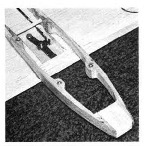
Ramin and Spruce crutch fitted to wing and tail and controls installed. Dural studs are for pan hold down bolts. Temporary balsa spacer at front used during construction.
