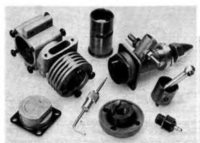
New addition to the ranks of British made sport engines, the Kingshire "Glo-Cat" 1.49, complete with silencer. Parts on left. Compared with diesel model, it has different piston, cylinder-liner, head, shaft and front housing.
