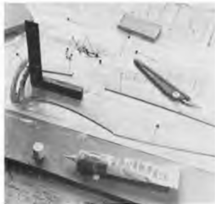
Assembly sequence for Sterling's "Zero" illustrates half keel construction. Above: half formers are added to outline frame. Below: when formers are in place main side stringers are added, before removing from board, adding second half of formers and remaining stringers and finally, vac formed nose cowl.
