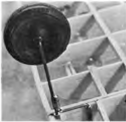
Left: Tube sockets epoxied in wing accept undercarriage legs, removable for flight.
