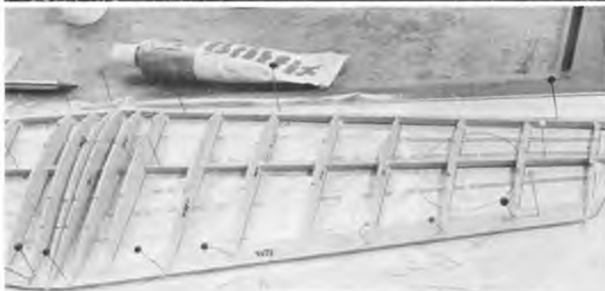
Above: Standard wing construction on Sterling's "Zero", note use of polythene sheet to protect plan.
