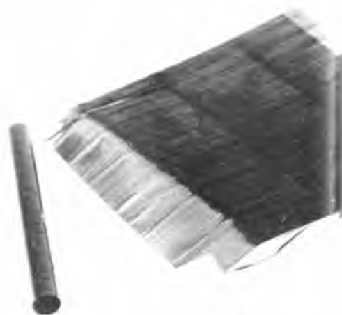
Epoxy impregnated fibres (right) which roll into tubes (left).
