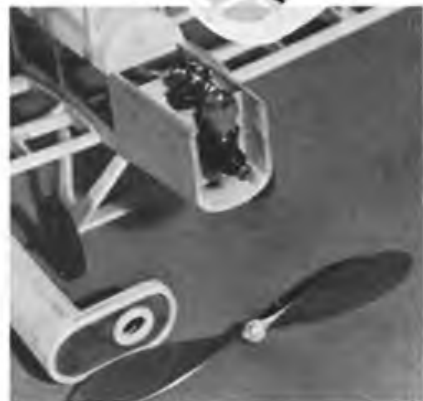
Humbrol CO 2 motor installed in nose of Comet's "Curtiss Jenny".
