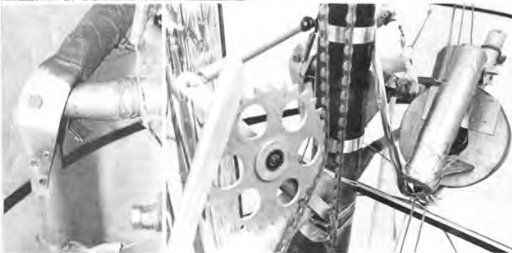
Left hand controls pitch and turn Right hand sets clickstop warp disc. Note plastic chain and sprung idler for chain slack.
