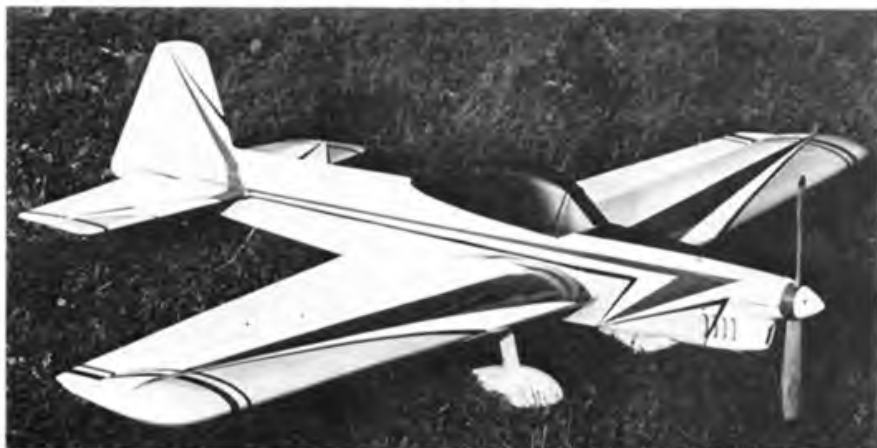
Above: Glen Alison's latest aerobatic model featuring Al Rabe aerofoil section wing including dihedral, powered by Super Tigre 46. Fuselage is covered in light glass cloth, finish is K&B Super Pox and all-up weight is a modest 45oz.
