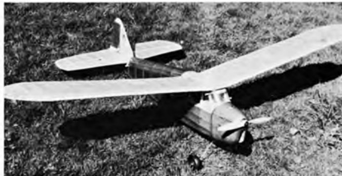
This 1948 Bill Winter Skybo built by reader Peter Miller was made from an American kit that came to this country via New Zealand! Model is R/C assist on rudder and throttle and is powered by an old 2.5cc Jena diesel.
