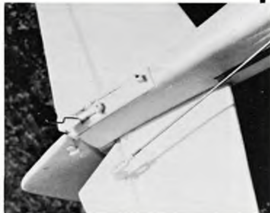
Right, tail assembly showing rear wheel fixing and adjustable control connectors.
