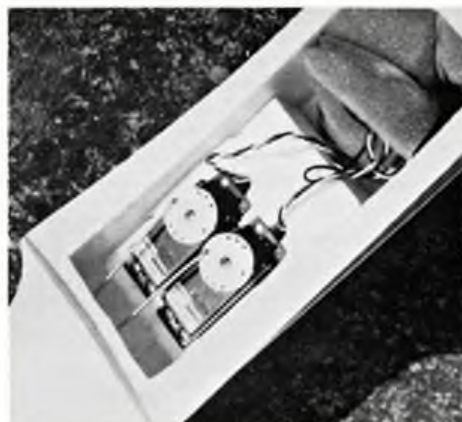
Right, three different size foam servo trays are supplied. The servos simply push fit in place, and the tray is glued in position after finding the correct location.
