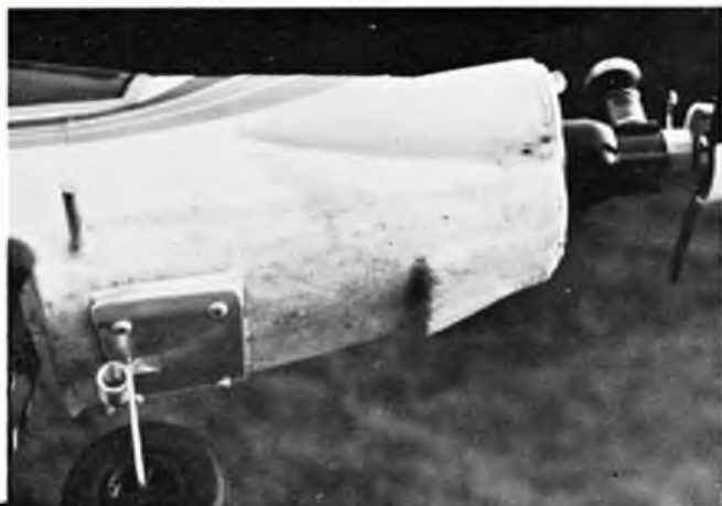
Right, repair using medical bandage and PVA glue.
