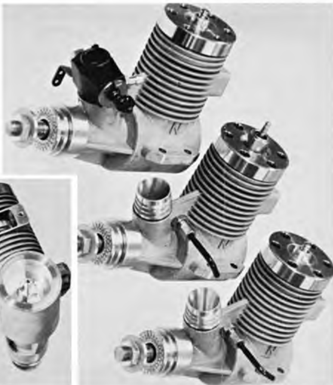
Right: three versions of the Nelson 15 engine from top to bottom: R/C type with FAI head, FF/CL model with plug insert head, and FF/Speed with FF head
