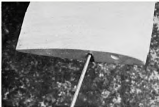
Left, shows the single 10 swg wire wing joiner. We did fit a ply face to the end of our wing, as the trailing edge corner is prone to damage.
