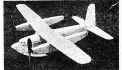
G.B.2 By H. S. Sayers One-time holder of the British Record for flying boats, this model employs a high wing mounting, and twin motors on a stepped boat type hull. Span 47 inches. WP/134 Price £2.95
