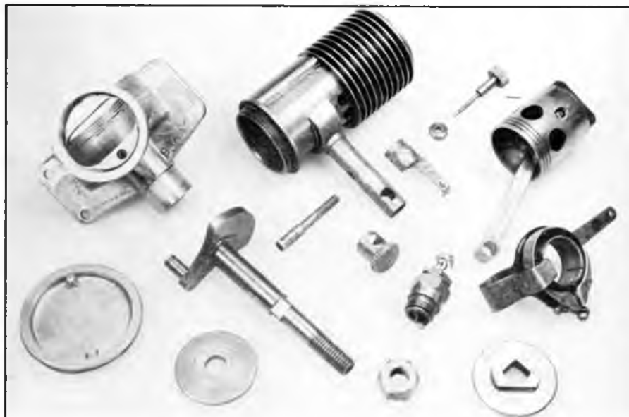
Outwardly, the low-priced Model D was identical to 'B' and 'C' except for simplified carburetor assembly.
