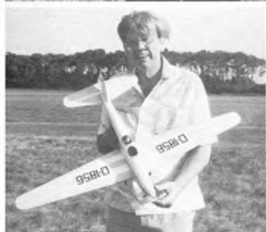
Arthur Evans never shrinks from the 'difficult' - his Gnospelius Gull demands 22g piano wire drive to twin props from the central rubber motor. Left Barry Hotham's bright blue/white B123 flies well, if unpredictable, from Model Builder plans. Top centre, 'Spirit of 1916' as Camel chases the Chas Newman Pup, a neat pair, and above Harry Perrens prepares to release his Rearwin Speedster, forever a nice kit subject with all the right proportions. Left, below: reappearing for its annual OW outing, this 'Prince of Wales' Airspeed Envoy is a show stopper if not exactly outstanding for its negative rate of climb. Yes, the plan (FSR 126) is still available on request, price £2.45 incl. post.
