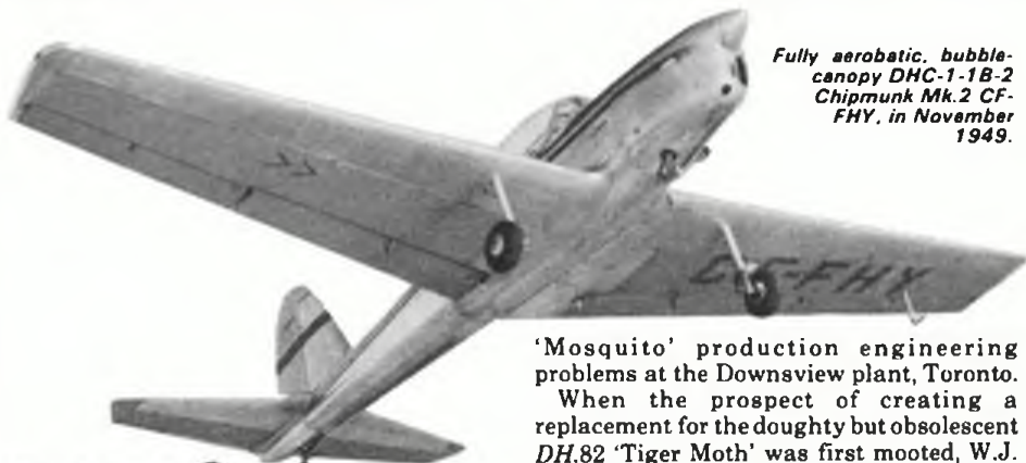
Canadian built DHC-1B-2, with Gipsy Major 10, full aerobatic clearance to 9g stress factor.
