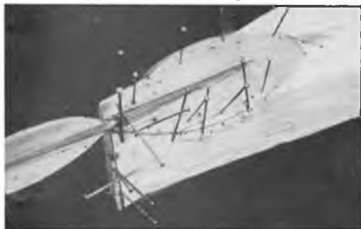
Plenty of pins used again as propeller pitch is "set". Note sticky tape and small wooden "Clamp" hold prop. shaft in position.
