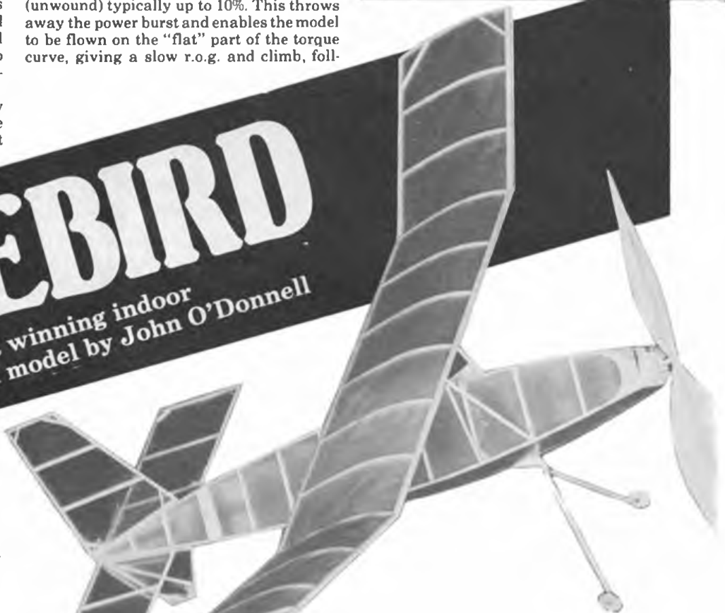
Top. Propeller assemblies and undercarriage. Very positive location using bamboo pegs on noseblock. Above, simple function lines of “Cagebird”, note wing braces on starboard side only.
