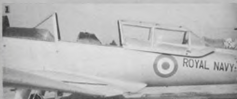
The De Havilland T.Mk.10 standard Chipmunk in close-up: 1 — showing fully open cockpit, 2 — dorsal fin and anti spin strakes, 3 — landing light only on port undercarriage leg, note root-stall inducing strip on wing leading edge, 4 — wing-root fillet and rivet pattern on fuselage, 5 — elevator trim tab on starboard side only.
