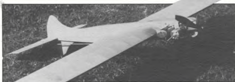
The simple lines and structure of the 'Easy' made it a popular model in the forties. This version powered by 5.3cc Valkyrie in R/C configuration but without throttle.
