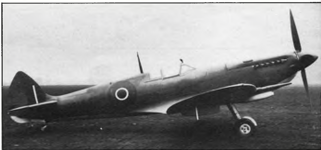
Above, echelon of four RAAF aircraft somewhere in Australia. Note overpainting of red roundel centre in white on first three aircraft (photo Jack Beaumont). Below, MD 319 - L.F. Mk VIII, early example with splined oleo legs.
