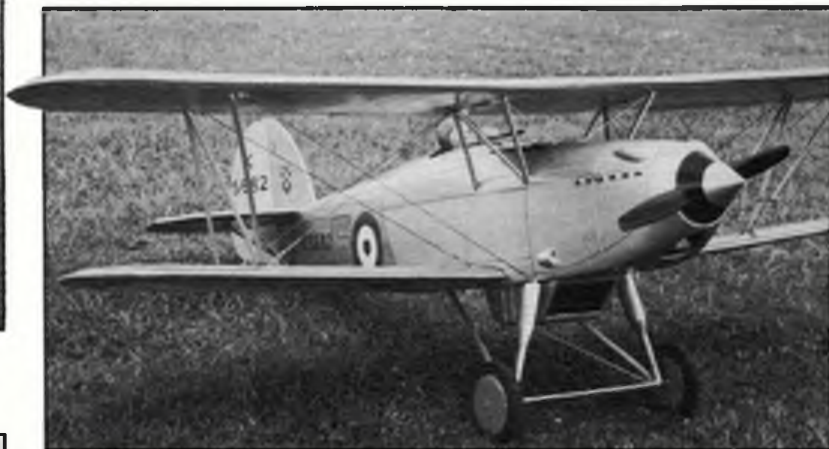
Above and right, Geoff Burkett's Hawker 'Fury', Merco 61 powered, covered in nylon and with a very realistic silver finish from car aerosol spray cans - he did not let on how many cans though!
