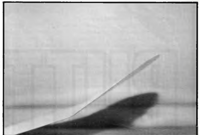
Above left: Before and after - a wing blank, shaped and marked into panels, lies in front of a finished example. Above right: Right-hand tip washout. Take care to get all trimming angles correct. Bottom left: A simple jig ensures accuracy. Note set-square, which is used in conjunction with lines marked on jig base. Bottom right: Quarter-grain wood is used for the butterfly tail. Button thread outline adds strength for negligible weight.
