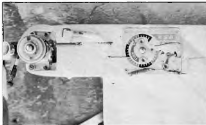
The fuel shut off system on Trevor Payne's 1/2A Slow Open model. He uses a modified DT-timer which he doesn't recommend as it is too erratic but the mechanics are super simple and allow a plate equipped timer to run on after fuel shut off. Spring loaded lever crimps down onto tube just behind engine.
