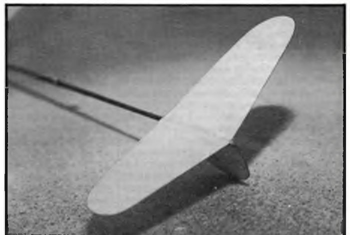
Above left: Before and after - a wing blank, shaped and marked into panels, lies in front of a finished example. Above right: Right-hand tip washout. Take care to get all trimming angles correct. Bottom left: A simple jig ensures accuracy. Note set-square, which is used in conjunction with lines marked on jig base. Bottom right: Quarter-grain wood is used for the butterfly tail. Button thread outline adds strength for negligible weight.
