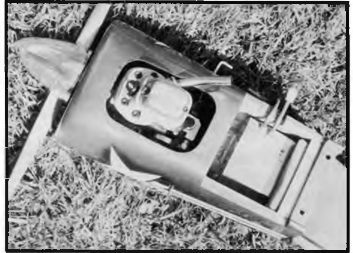
Engine accessibility is excellent; there's plenty of room to get at everything. Not much room for the tank, though. It's held with foam rubber at the rear. Note the little pin on the left side of the nose - it's a trigger for a home-made choke system.
