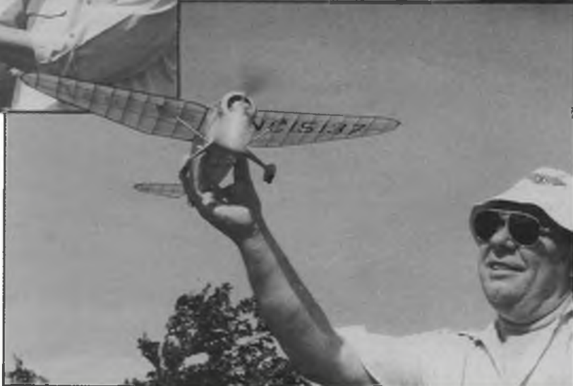
Above: This Douglas O-38 (a Ken McDonough design) flew well for Phil Brooks, who had to keep the turns down on the windy conditions at Old Warden. Above right: Rudders in the propeller slipstream of his H J Townner designed Hampden will, hopes Colin Young, reduce the directional stability problems that afflict single-rudder rubber-driven twins. Plans (first produced in May 1941) are still available from Authentic Scale of Eastbourne. Right: Harry Perrens of Walsall with his nicely-made Comet Stinson Reliant.
