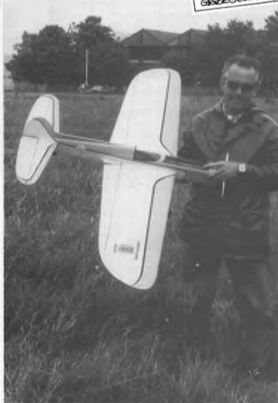
John Kergon favours the APS Superhawk, Bill Draper's winning design. Super Tigre 46 power - and CLAPA decal on near fuselage!
