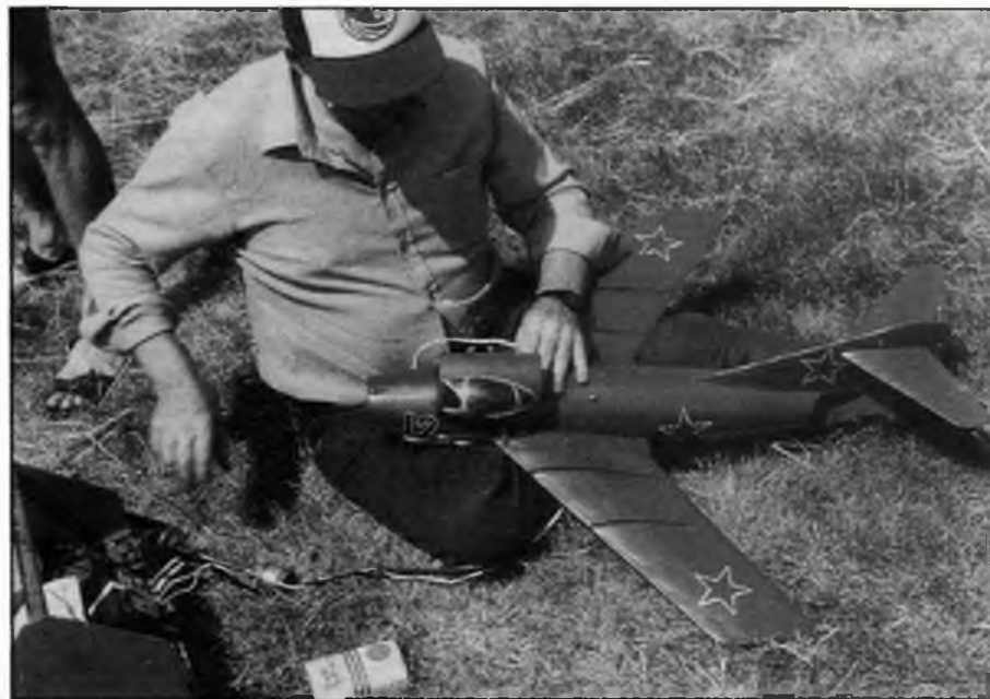
Top: This PE Norman-designed MiG 15 by Alan Campbell has a highly efficient home-made impeller and ample thrust to fly well. The lack of windscreen allows even more air to enter the fuselage. Above: Alan reaches for the starter motor with its extension shaft the MiG's OS FSR. 15.
