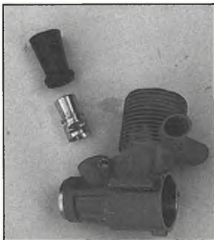
Bare crankcase with venturi and rubber muff. Venturi is inserted into muff; assembly is pressed into crankcase boss. Spraybar is then pressed into place to fix the lot.
