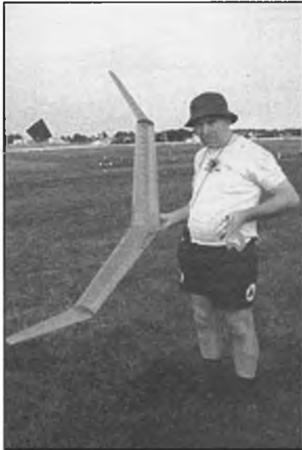
John's 6ft Tailless Glider, originally designed on a sheet of school graph paper in 1948, was built in 1983. Consistent half-minute flights.
