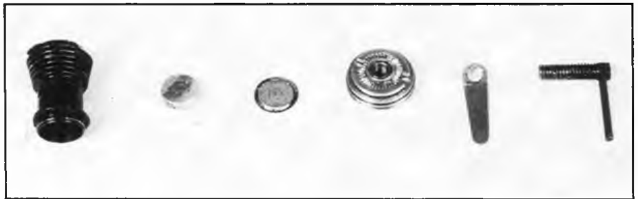
Easy – all you need to know in exploded form, above. Photo below shows Pee Wee cylinder; new contra-piston and diaphragm; Pee Wee head bushed for compression screw and locking lever (shown at right). News of similar experiments welcome!
