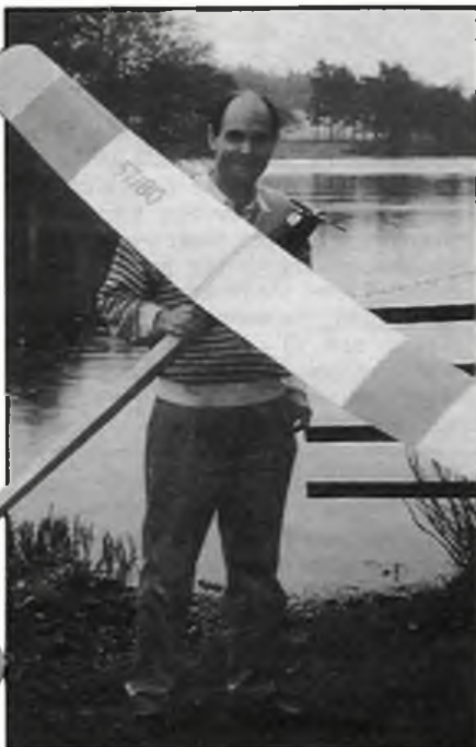
Even further development has produced this Open Power design. Techniques used for wing and tail described in text. 80in. model weighs 40 oz; could easily reduce by five ounces. Yet to come - a 100in. version for piped K & B 40!
