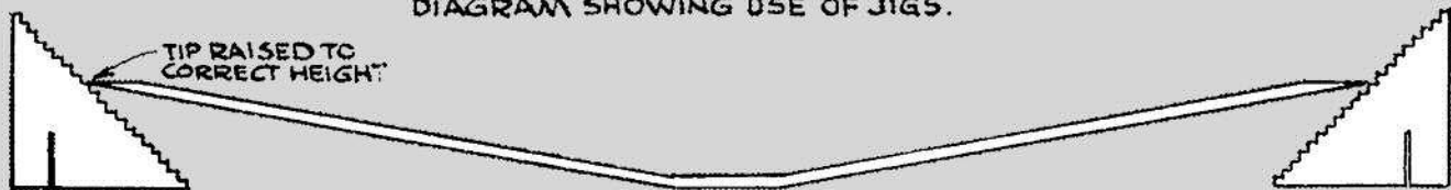
DIHEDRAL ANGLE INCREASED BY WING TIPS BEING PLACED ON HIGHER 'STEPS'.
