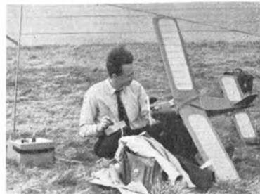
E. Kreulen's (Holland) latest receiver is 3 valve, modified from an Honnest-Rodlich circuit. Has so-called positive feed back, 3 m/4 rise from zero. Range is 5 kilometres on test; 2 watt Tx. Valves, DC30, 6B6, and 6L6. Transmitter must be tone modulated. Typhoon escapement in foreground. Below, Jan Hakke, first Danish radio control champion
