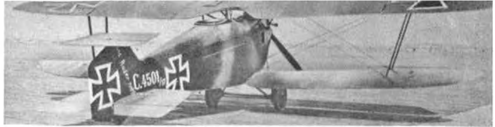
Prototype Hannover CL II. Note angular upper tailplane and uniform dihedral which distinguish from production aircraft. Lettering on rudder is a "hands off" note
