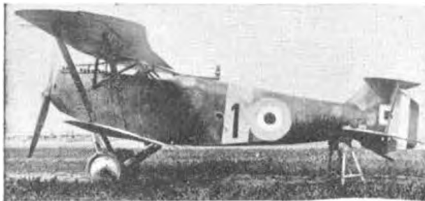
Above, captured CL IIIa displays late 1917 type serial number also tailplane bracing struts which were later removed. J.W.M. Photograph Q 57638. Right: Uncamouflaged machine built by L.F.G. (Roland). It was designated CL IIIa by this firm but was in fact a standard CL IIIa
