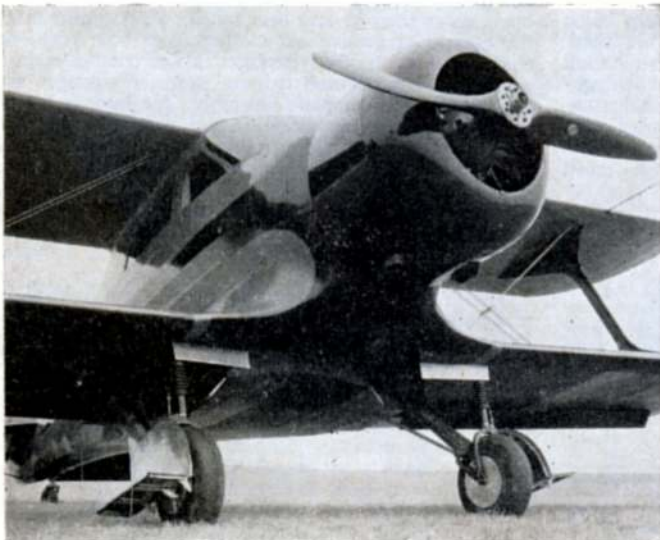
Beechcraft factory photo dated February 23rd, 1934. Model not identified, but almost certainly a B-17L. Note the early arrangement of undercarriage doors.
