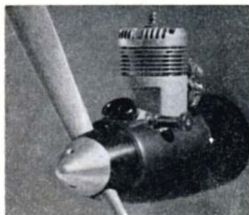
The horizontally opposed, simultaneous firing twin cylinder "Duo 29" 5 c.c. diesel from Robbe in Germany features a radial mounting to allow for the overhang of rear shaft induction. Throttle has Amal style action with needle valve moving within the air choke. Cylinders are reminiscent of the Zeiss Activist 2.5 c.c.
