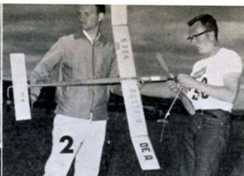
THE WINNER (photo 5), Joachim Loffler of East Germany preparing his better model for the fly-off. Uses taper wings and tubular fuselage in contrast to squared-up reserve. Power is 18 strands of 3/16 in. Pirelli (580 turns) for calm weather or 20 strands (480 turns) in wind. Prop is 22 by 23½ in. twin folding blades, on a ball race supported shaft. Model has light yellow tissue finish, long tail moment and small tail area
