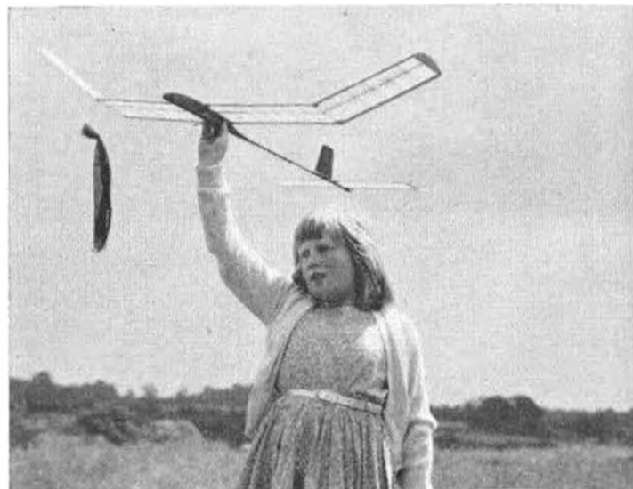
Figure 6.2. How to hold a model ready for tow launching. Miss Barker is supporting the "Downbeat" A/I design described and drawn in last month's feature with the towing ring hooked over the launching hook on the model, and the nose held slightly upwards in order for the model to "kite" into wind as the launcher begins to run into wind.
