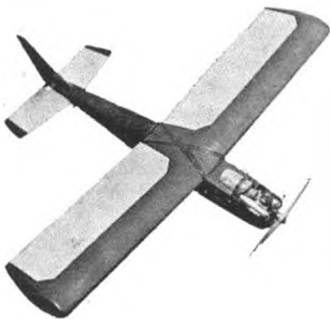
Rugged lines and swept fin are clearly shown in this view of Bazz Bomb . Note the O.S. Jetstream silencer on the O.S. 15 R/C. Model was very fast on this engine and 1.5 c.c. should be the maximum power limit for initial flights.
