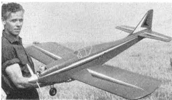
Below, one and a half times enlarged "Pylon Duster" by Dennis Helford, modified with dorsal cockpit and reshaped fin with Merco 49 and F & M R/C gear seen with S.M.F. club.
