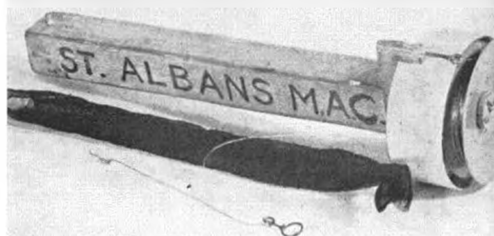
Figure 6.5. A self winding, rubber driven winch, as sketched in Figure 6.4, and used by the author. This type of winch was originally devised by Cyril Mayes one time member of West Essex Aeromodellers, now a resident of Canada. Simple square balsa tube holds the rubber motor which returns the line automatically after it has been paid out.
