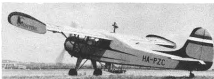
Hungarian PZL101 Gawrons go through the alphabet from PZA to PZZ and then in to the PXA-PXH series. All yellow with black trim, later versions differ slightly with cowling scoop. Note hopper and spray bar versions.
