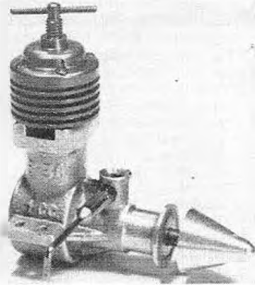
Above top, the new McCoy "Custom" stunt .35. These McCoy models are now fitted with hard chrome plated pistons. Above, the Barbini 1 cc. looks rather "thin" by modern design standards.
