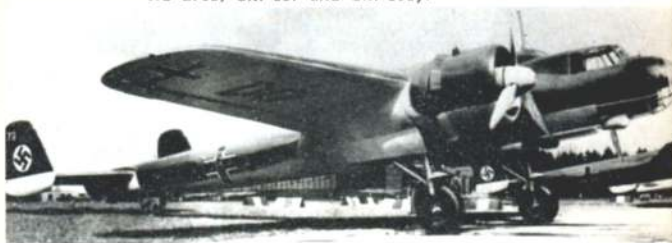
Above: Early production Dornier Do 17Z-1 with Bramo Fafnir 323A-1 engines. The Luftwaffe started to convert to the type early in 1939. Note the two-tone green splinter camouflage – and the highly polished natural metal propeller blades. Below, top: A Dornier Do 17P with the rounded shape nose, bearing number 73 on the rudder and 73 superimposed over a 25 marked centrally on the fuselage cross. This version has BMW 132 N engines. Below centre and bottom, two views of a Yugoslavian Air Force Do 17Ka surrendered in Egypt. This version was made under licence by the Yugoslavian State Aircraft factory; the badge of which is seen on the fin. Note very small insignia above wing, near tip, and larger insignia on the underside. (I.W.M. Photos HU 2703, CM 697 and CM 698).
