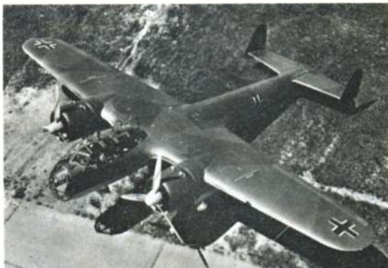
Above: Early production Dornier Do 17Z-1 with Bramo Fafnir 323A-1 engines. The Luftwaffe started to convert to the type early in 1939. Note the two-tone green splinter camouflage – and the highly polished natural metal propeller blades. Below, top: A Dornier Do 17P with the rounded shape nose, bearing number 73 on the rudder and 73 superimposed over a 25 marked centrally on the fuselage cross. This version has BMW 132 N engines. Below centre and bottom, two views of a Yugoslavian Air Force Do 17Ka surrendered in Egypt. This version was made under licence by the Yugoslavian State Aircraft factory; the badge of which is seen on the fin. Note very small insignia above wing, near tip, and larger insignia on the underside. (I.W.M. Photos HU 2703, CM 697 and CM 698).
