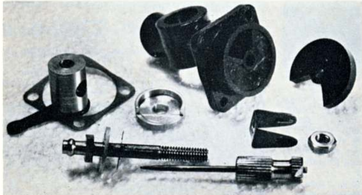
Above: Parts of the E.D. Super-Fury R/C rotary-valve and carburettor assembly. Complete unit is interchangeable with standard type.
