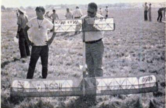
Top: George Perryman, Smyrna, Georgia. A threat in any rubber-powered event. Flew Unlim. Rubber, Wake, Coupe d'Hiver. Trademarks are swept-back wings, polyhedral stab, checkerboard covering and scimitar tips on everything—including the prop. Doesn't seem to hurt the performance any. Took second in Unlim Rubber. Assisted by Mike Bailey who took first in Sr Unlim using Perryman design. Above: Vic Cunningham, Jr., Covina, Calif. Manufacturer of popular Galaxie and Geodetic Galaxie kits for 049-051 engines. All designs in last five years have featured 'Union Jack' type of geodetic construction. B and C models are K & B Torpedo-powered.
