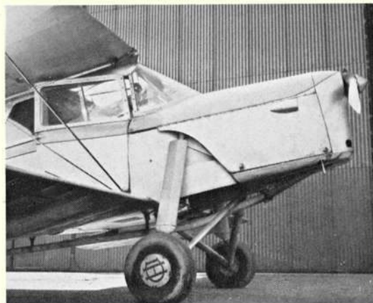
De Havilland monogram on the wheel cover should not be overlooked by modellers. The fairing over the undercarriage oleo strut can be turned through 90° to act as a surprisingly effective air brake, as will be appreciated by comparing this photograph showing the width of the fairing and the photo below which illustrates its thickness.
