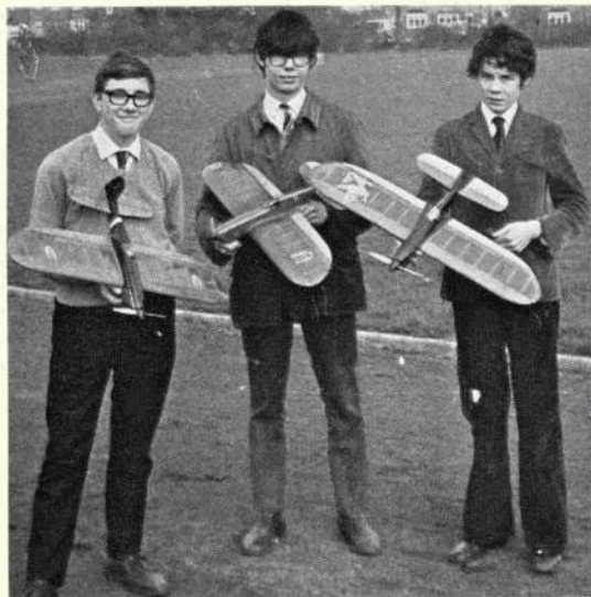
Three more Reactions built by members of the Allerton Grange School model club. All the models have been constructed to a very high standard, which is well rewarded by the resulting high performance. Weight must be kept down so use coloured tissue for the wing coverings in lieu of a heavy paint scheme.
