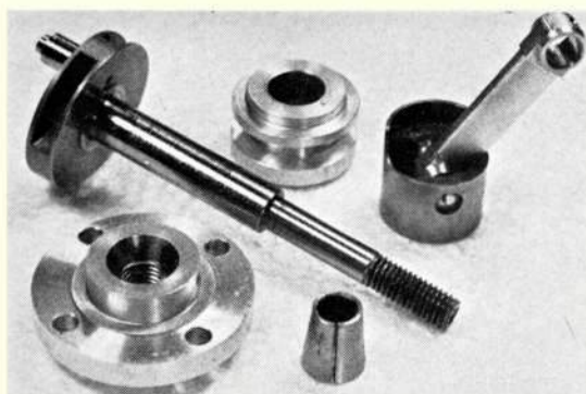
'Start' shaft has peripheral counterbalance slots without sealing rim. Note extensively cutaway piston skirt. Con-rod shank is oval section.
