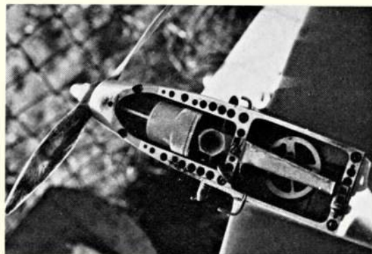
Neat installation of Hasling's HP15 motor in his team racer. Extensively lightened crutch mounting was made by his brother. Note circular bellcrank employed - also lightened. Complete model weighed just over 19 oz.
