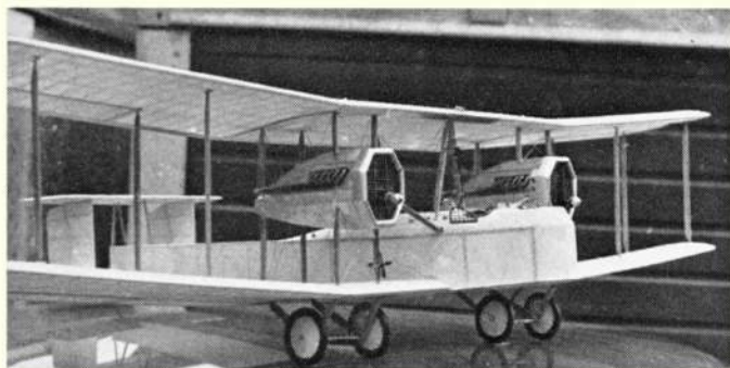
The latest Manley creation is most ambitious, a Vickers Vimy Atlantic, utilising two Mills .75 c.c. engines, and to approximately 1/16th scale. Model painted overall with magnolia emulsion paint, while the cowlings are once more chemically etched aluminium. Twin engined free flight scale models are not for the inexperienced or weak-in-heart!
