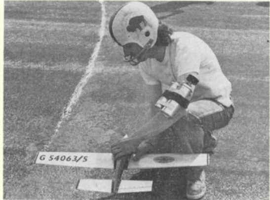
John Daly runs up his diesel-converted K&B 15 Schneurle port engine prior to a heat. Protective head-gear is both compulsory and sensible - John's stylish 'tiff'er' being originally designed for ice-hockey players!
