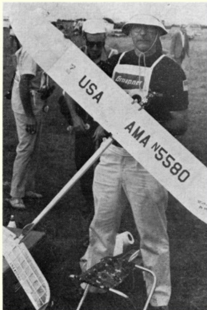
Left: Bert Huijben of Holland was another to drop in the 4th round, spoiling an otherwise perfect record. His all-sheet surfaces and tubular fuselage with the almost universal Rossi 15 for power is typical of Western Europe, while at right, Tom McLaughlin of the U.S.A. showed experiment. Tail is swept for extra moment without fuselage weight, and wing swings on pylon for climb/glide trim washout control. Tom lost just one second on last flight to miss the fly-off and placed an unlucky 13th!
