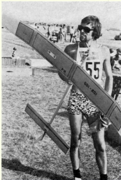
Left: Bert Huijben of Holland was another to drop in the 4th round, spoiling an otherwise perfect record. His all-sheet surfaces and tubular fuselage with the almost universal Rossi 15 for power is typical of Western Europe, while at right, Tom McLaughlin of the U.S.A. showed experiment. Tail is swept for extra moment without fuselage weight, and wing swings on pylon for climb/glide trim washout control. Tom lost just one second on last flight to miss the fly-off and placed an unlucky 13th!
