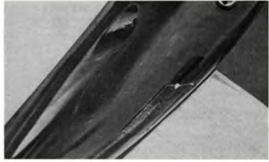
When retracted, the underside of Krasnorutsky's team racer presents a very 'clean' picture. Unit retracts under centrifugal force, extends on operation of the engine shut-off i.e. when sharp down elevator is applied. Several top teams are now working on similar devices.
