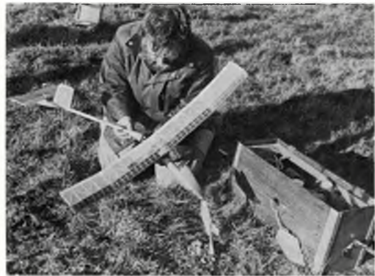
Detaching the rear fuselage boom gives access to the rear motor peg for winding. Note the size of the model box in the foreground – two models plus all associated flying equipment packs into that small container!
