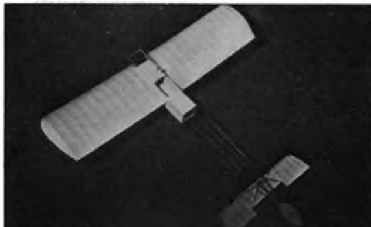
Clyde Cessna's 'Blériot' - very like the first aircraft 'Peanutted' by Butch Hadland with basswood longerons and all bracing.
