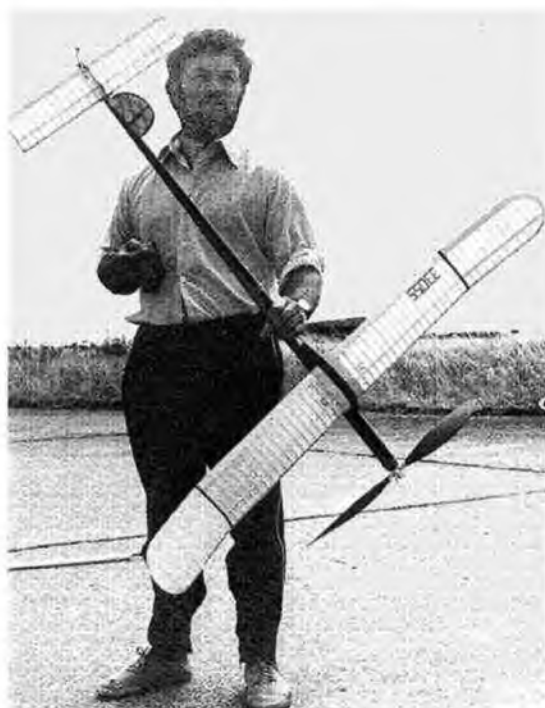
Welshman John Bailey and Wakefield with alloy prop hub, two piece wing and fuselage, built while he was teaching in Zambia. one pence piece (3.2g) – remains at a low level, hence the minimal entry in Pennyplane at the Nationals.
