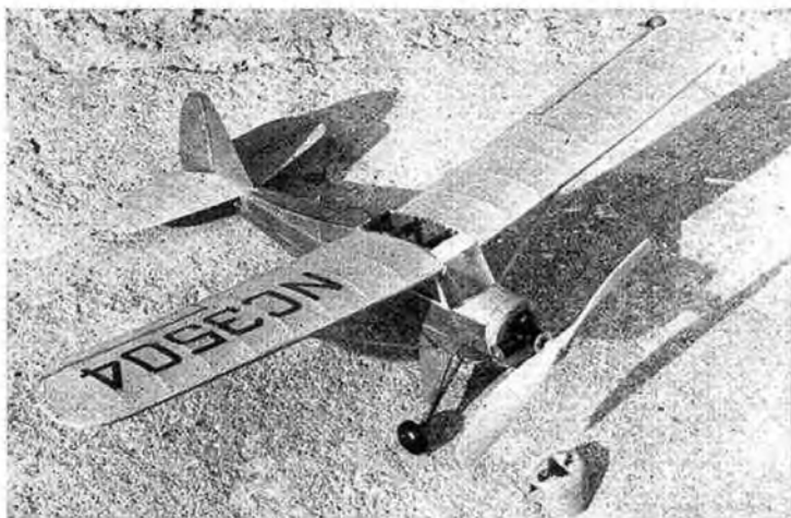
Another view of the Tern Porterfield Collegiate, very simply converted from rubber to CO 2 power by the addition of a ply firewall, and the Telco unit retained by a pair of bolts. With the motor mounted on its side, not only was the thin copper pipe protected, but downthrust could easily have been adjusted by the addition of washers beneath the mounting lugs. Sparklet CO 2 bulbs can vary enormously, thus exact power comparisons are impossible.
