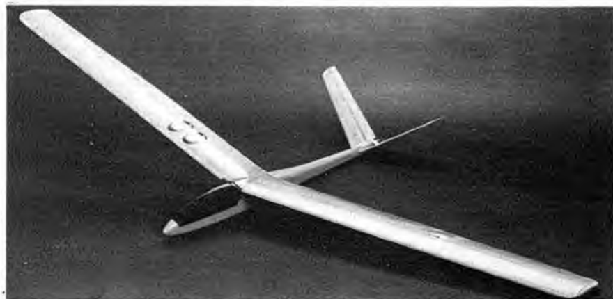
Above: Butterfly tail emphasises the elegant silhouette of this super simple RIC glider. Although primarily designed for slope flying, excellent glide also allows flat field flying, especially with the larger 2400mm span wings.
