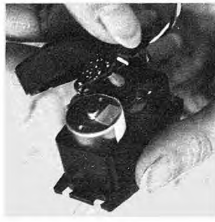
Right: With all screws removed carefully open plastic case, taking care not to break or strain wires or damage internals.
