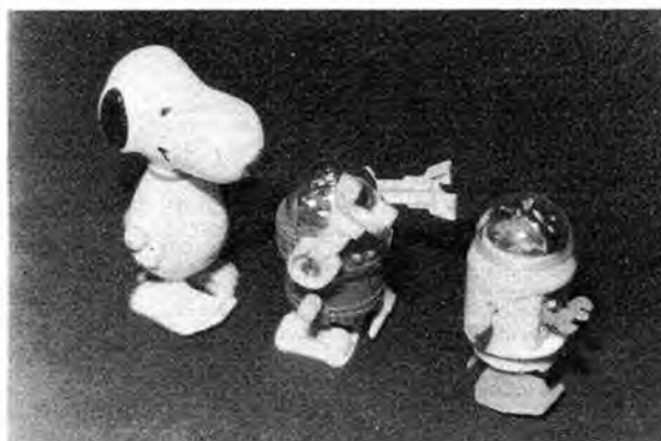
Top: lightweight nylon clockwork timers, weighing from 2.2 to 3.7 grammes each, are to be found powering walking toys made in Hong Kong currently on sale in most toy shops, as illustrated left.
