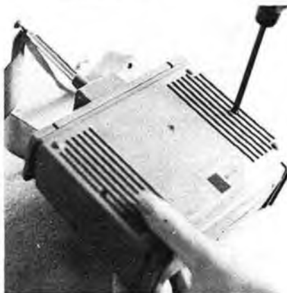
Right: Use cotton wool swabs moistened with a little methylated spirits to carefully clean all contacts, not forgetting one in centre.
