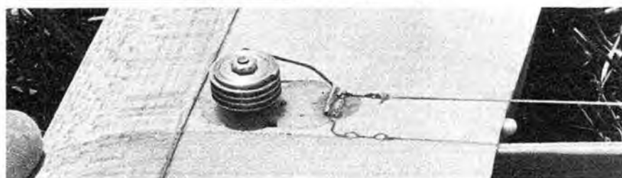
Below: One such timer shown mounted in the wing of Edward Liem's all-sheet balsa chuck glider wing, fitted with Seelig F1B Wakefield scroll to permit several revolutions during run-down to D.T. Bottom left: underside shows hold-off pin running through aluminium tube sandwiched under throw tab exiting at trailing edge. Bottom right: tail end shows 50% chord span-wise hinge line and small wire coil spring to activate D.T. elevator.
