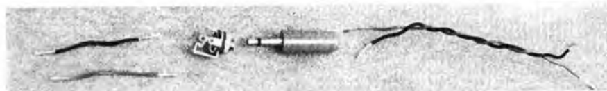
Above: Remove back of transmitter, usually held in place by two small screws. Above right: Start by drilling hole in transmitter case to suit diameter of jack socket body being used. Below: Jack socket with plug which can be fitted to case of transmitter permitting simplified recharging with ni-cad cells left inside transmitter. Right: Carefully wire the socket into the existing battery pack circuit, paying particular attention to polarity of wiring. Bottom left: Modifications completed, show external jack plug used for charging, fitted to socket mounted in transmitter case. Bottom right: Alternative modification on this Sanwa 2 equipment uses charging socket added to battery pack which simply tucks inside transmitter during use.
