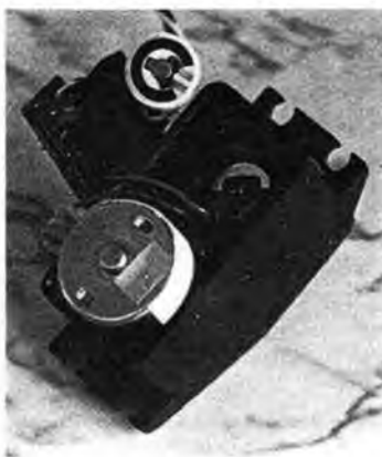
Far left: Mark the position of the potentiometer with relation to case using Biro or pin scratch before loosening two retaining screws.
