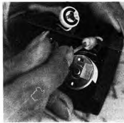
Right: Use cotton wool swabs moistened with a little methylated spirits to carefully clean all contacts, not forgetting one in centre.
