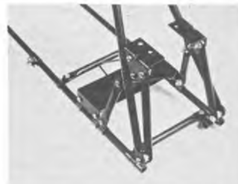
Right wheel mounting. I glued the P clips to the tube of the fuselage with Cyano, as they tend to move with a hard landing. Left, the wing centre mounting. Below left the components of the kit straight out of the box. The servo mixer can be seen below. This gives up and down and aileron control via the two push/pull rods.
