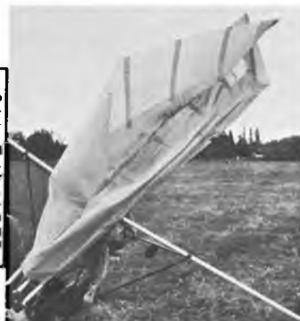
Right: wings folded for transportation; if the wing spars are removed the model takes up very little room.
