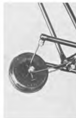
Right wheel mounting. I glued the P clips to the tube of the fuselage with Cyano, as they tend to move with a hard landing. Left, the wing centre mounting. Below left the components of the kit straight out of the box. The servo mixer can be seen below. This gives up and down and aileron control via the two push/pull rods.
