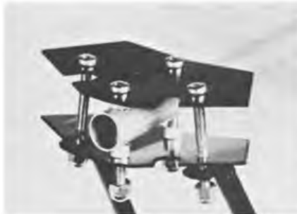
Right wheel mounting. I glued the P clips to the tube of the fuselage with Cyano, as they tend to move with a hard landing. Left, the wing centre mounting. Below left the components of the kit straight out of the box. The servo mixer can be seen below. This gives up and down and aileron control via the two push/pull rods.
