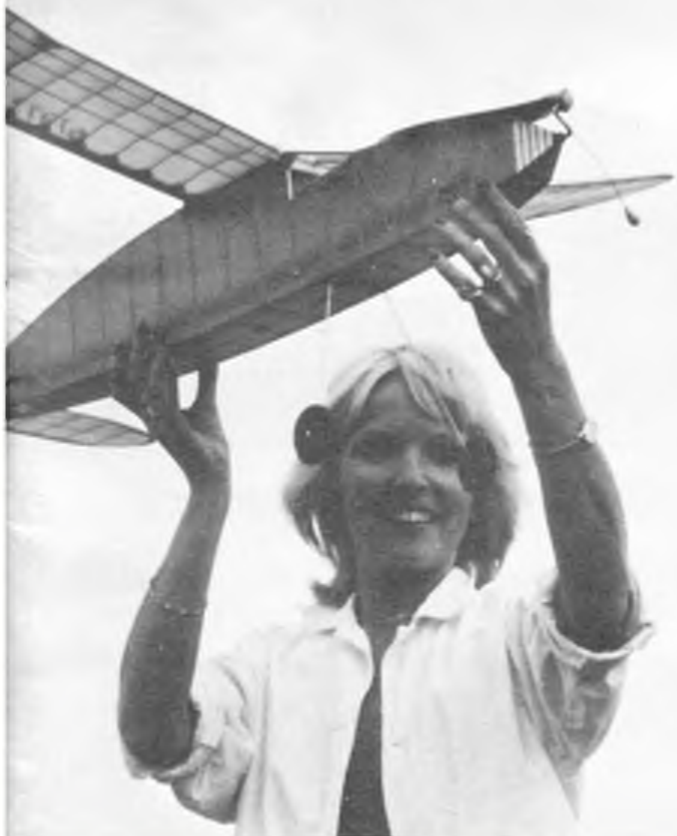
It is a replica of the famous F. J. Camm's 'Advanced Compressed Air Monoplane'. Span is 66in. Built from spruce and ply. Pine prop. 16in. dia. Dave (who is a S.A.M. member) adds that the tank is 5-thou. brass foil, tested to 150 p.s.i.!
