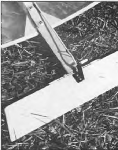
Left: Titov (2nd) fuels Doroshenko's Combat model before bout with Shiavato (Italy). Below: detail of tail on Doroshenko's model. Trailing edge from three laminations of 4.5 x 1.5mm spruce. Right: overall view of Doroshenko's model. Engine mounted on light alloy angles locked onto hardwood centre section insert.
