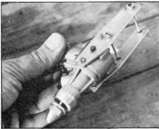
Left: typical combat engine mount system using previously mentioned aluminium alloy rails. Rossi engine shown here belongs to Leif Goransson (Sweden). Right: foil covering (also on Goranssons combat model) prevents rear exhaust from burning model.
