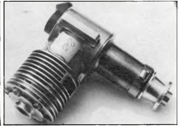
Above: note the boost port prime tube on the Kramerenko motor, just below cylinder fins. Left: carb. valve in-situ in winning model. Unconnected pipes are assumed to be overflow and vent. Below: twin forward facing exhaust ports on Kramerenko engine.
