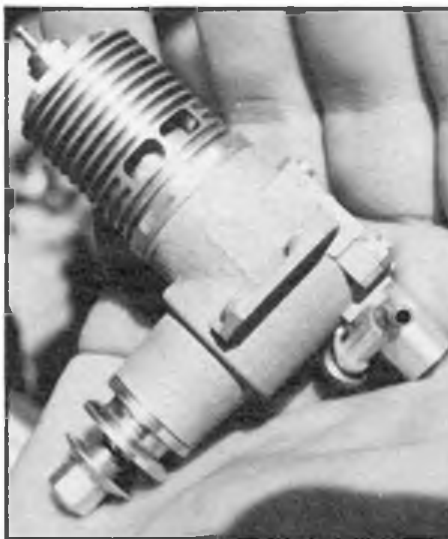
Below: latest combat motor from Doroshenko strongly reminiscent of 1948 Arden O.199. Drum valve, intake is in an unusual position. Note sand-cast finish to crankcase.
