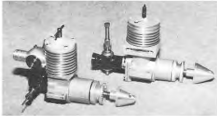
Hunter' 3.46cc twin ball-race, rear exhaust, and the MkII 'Viking'. The latter is a twin-stack side exhaust
