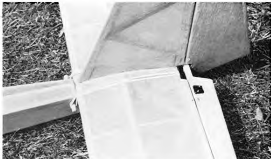
Below: detail of the tailcone showing the simple rudder and elevator controls.
