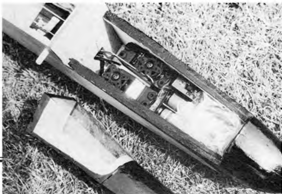
Above: Close-up of the Kestrel nose section showing the two-channel Sanwa radio installation. Note the battery box in the extreme front ahead of the two servos. Receiver is installed further back under the wing seat, just behind the main bulkhead.
