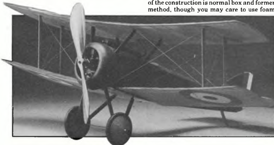
This view of the 'Pup' clearly shows the rigging wires, see text for their use as a trimming aid.
