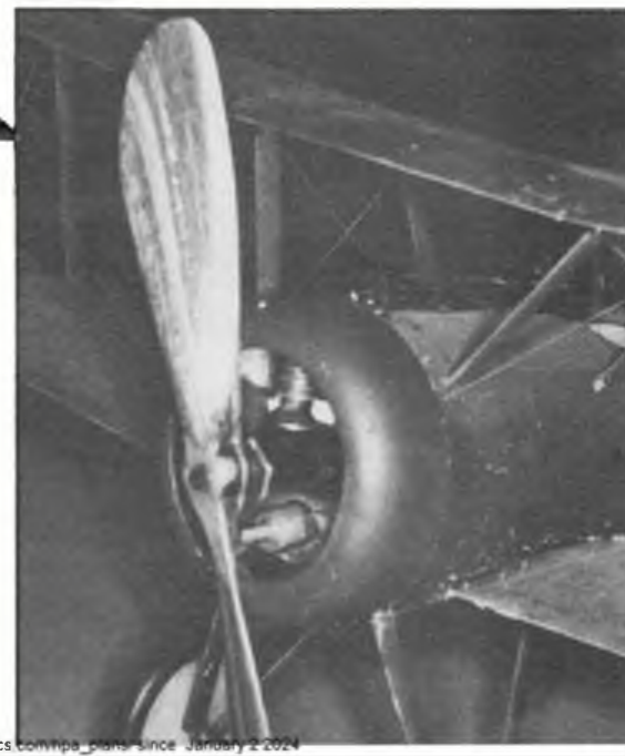
Close-up of the engine bay, sensible use is made of the engine bulkhead to mount the filler valve.
