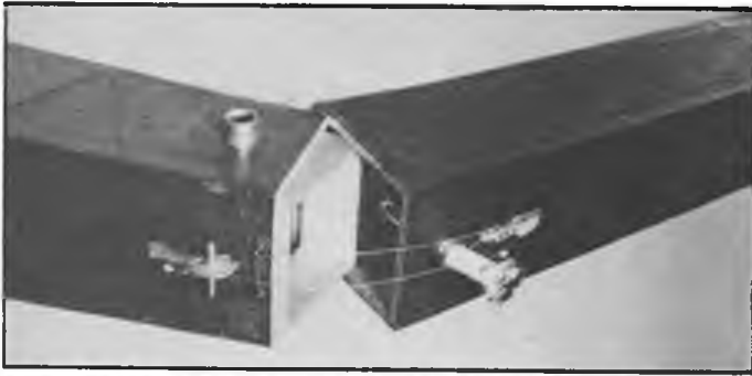
Derl Morley's Open Rubber model features the not often seen, hinging fuselage dethermaliser. Location of rear end must be very positive to ensure consistent trim.
