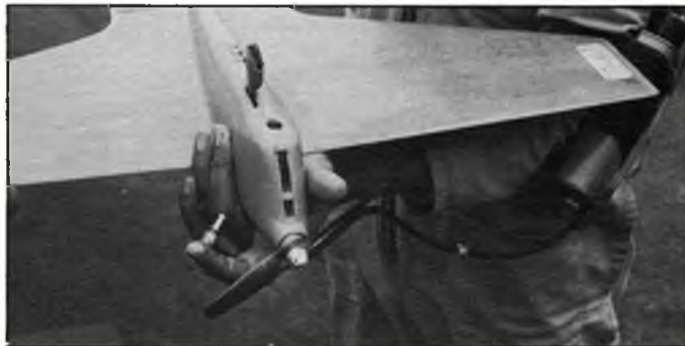
Left, 1976 World Champions Barkov/Suraev (USSR) - the team that had the best model but nothing to celebrate... Above, the lengths some people go to, to get the cooling right - the Van Uden brothers (Holland) show vanes everywhere on their typically Dutch flying wing.
