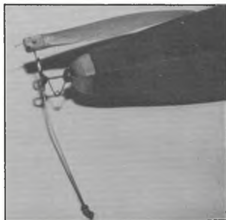
The prop assembly is a simple affair. There's only one blade to carve - what more could you ask!
