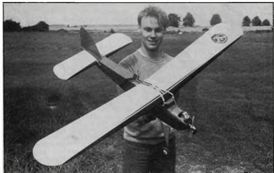
Small picture, opposite page: Simplex at rest. Made from the Aeromodeller free plan and powered by a DC Merlin, this model, fitted with Galloping Ghost type pulsed rudder operated by the Mattel transmitter shown here, was built and flown most ably by Mike Parker of Oxford. Far left: This flying wing, designed by Bernie Gross in 1947, was the result of much experiment in this field dating back to pre-war days. The eight-foot span beauty shown here was built for R/C - assist by John Wilkins of Chesham. The craft was featured in the January 1948 issue of Air Trails, detail from which appears at left. Model was described as 'a successful flying wing'. This page, top: Tony Harper of Newmarket with his yellow and white Northern Star, a pre-war Bob Copland design of 38 inches wingspan. Centre left: Ken Tansley displays his Caribbean Grey Junior 60. The initials on the tail surmount one of his few remaining original Northern Heights club transfers. Model is PAW-powered; note the natty exhaust pipe leading from the transverse silencer. Tubes emanating from the top of the rear fuselage house the 'snakes' which impart movement to the control surfaces. Centre right: Don Knight with his Earl Stahl Wayfarer, a model that made its first 'public' appearance at last year's SVAS Model Day. A stall near the ground at this year's function telescoped the forward fuselage with the result seen here. Model is or was, before damage, a great flyer; one of the best performing Earl Stahl designs. Above: Chris Knight with his un-named CEB Practical Mechanics Vintage Style model. Its ME Heron was a reluctant starter but problems were overcome and the model later flew well.
