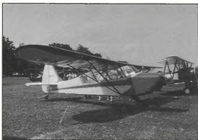
Trio of illustrations above relates to Interstate L-6 discussion in text. Aircraft of the Fighting Powers drawing, used by John Watters to produce our full-size L-6 plan in the August '86 issue, gives no clue to outwardly-sloping cockpit windows but Jim Alaback's photos of preserved yellow-and-blue N48427 at Oshkosh reveal all. Below: Soft Hong Kong scenery forms a gentle background to Noel Stephenson's latest scale stunter, a Miles M.20 for 1.5cc motors. Soon to be an Aeromodeller full-size plan, this attractive version of the 'ten-week fighter' - that's how long it took to design the real one! - will augment Noel's Splitfire Stunters which appeared in the March issue.
