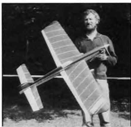
Walter Weineisen from Austria. Apparently conventional model has two-piece wing, carbon spar and engine cut-off.
