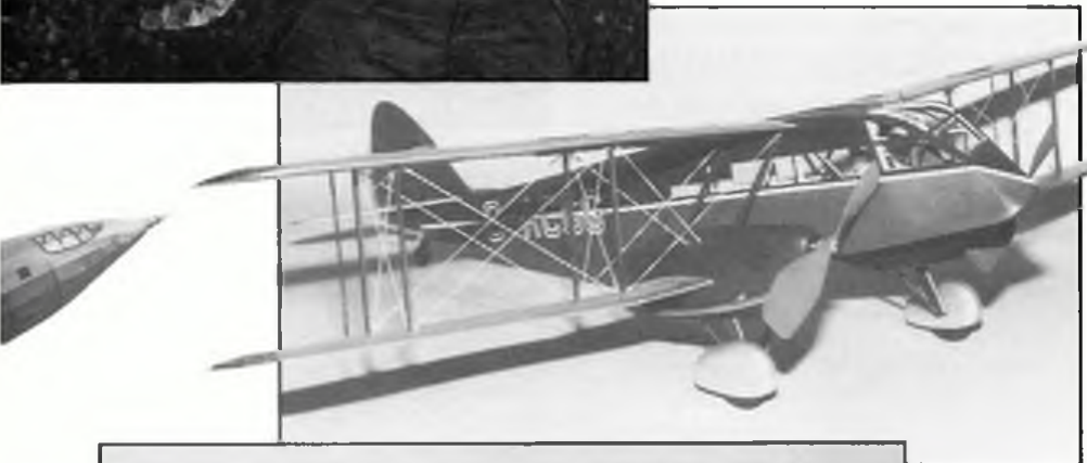
Below: Our reporter's DH Dragon runs on twin Brown CO 2 motors with three tanks plumbed together. 33in model won the Earl Stahl Trophy for best model. Bottom: Dennis Norman entered this Ju 88, successor to his well-known Lancaster (which still gained fifth place in Jumbo Scale).
