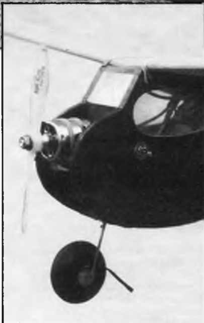
Above: Chris's own 32in, 250 gm Pee Wee. Direct drive M3 motor turns 5.1/4 x 3 prop; close-up at left. Four 180 maH cells used. Below: Field charger, as per circuit in Fig. 1, uses 6 x 1.2 aH 'buggy pack' to charge at 1.5amp.
