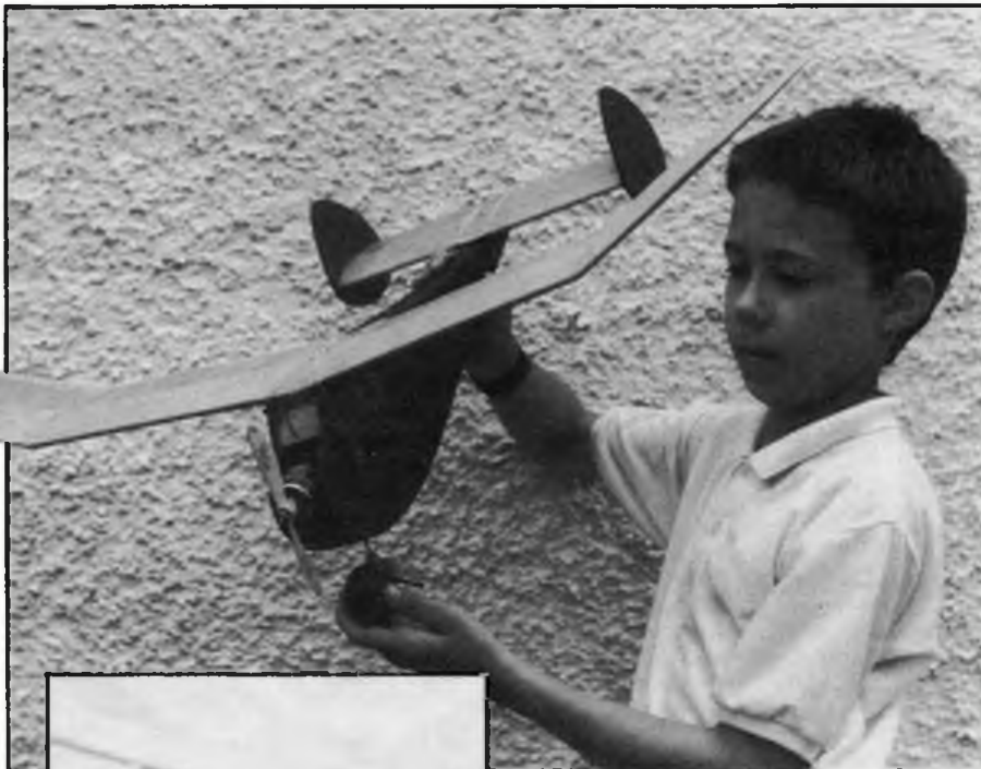
Above: Chris's own 32in, 250 gm Pee Wee. Direct drive M3 motor turns 5.1/4 x 3 prop; close-up at left. Four 180 maH cells used. Below: Field charger, as per circuit in Fig. 1, uses 6 x 1.2 aH 'buggy pack' to charge at 1.5amp.
