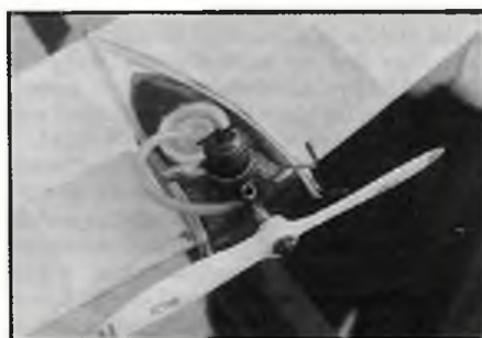
Motor detail shows simple mounting, fuel tank from 35mm film canister and DC Dart with exhaust collector ring, a one-time DC accessory.
