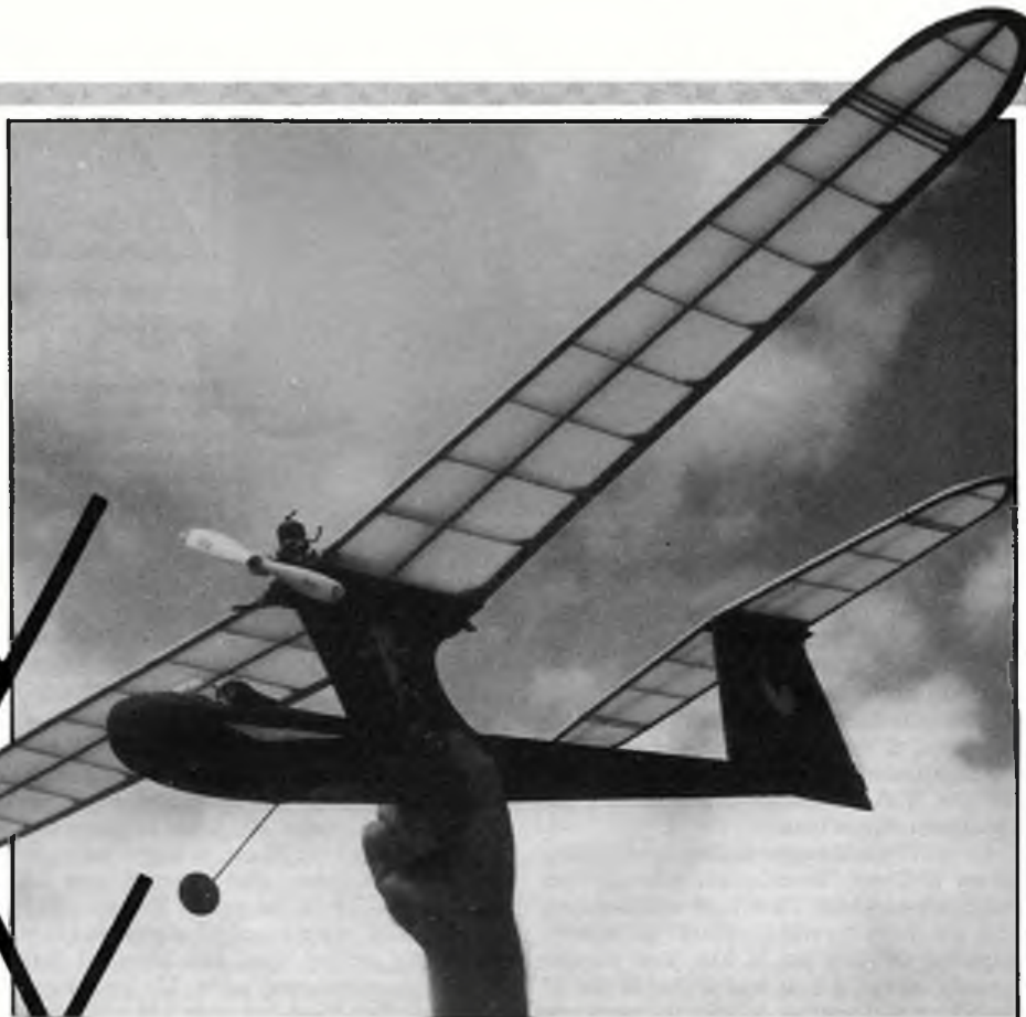
Vic Smeed's forty-eight-inch powered-glider style free flighter for motors up to 0.8cc
