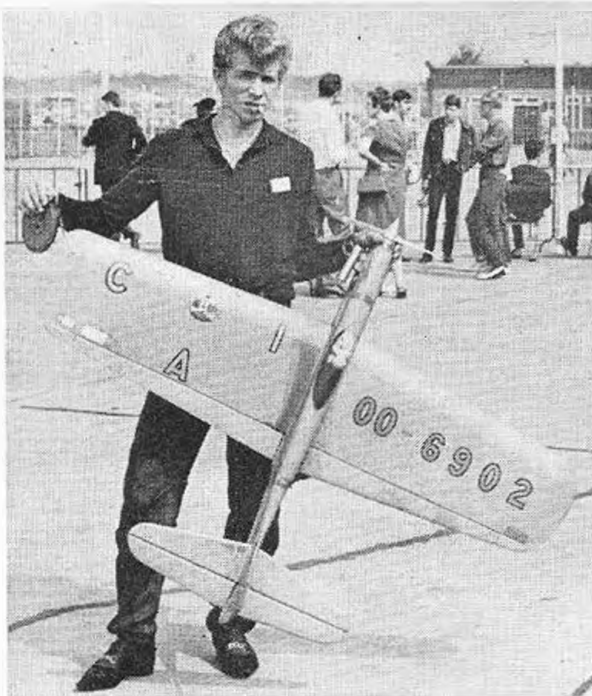
Above, Milan Drazek's new M.V.V.S. R.L. 15 team racer. This has the best finish we have ever seen on a team racer and is fuelled via a pressure system on the mechanics arm. Left, Stunt winner M. Vanderbeke of Belgium the host nation for the Criterion. He excelled with his second round flight with this silenced model and restored to the Belgians an International Stunt win. They used to dominate this event.
