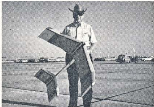
How's this for a swept wing? Roger Mason, who comes from Kansas calls his design the 'Swope' and uses it for two classes. A Super Tigre .15 is fitted for class 'A' and a Super Tigre .23 for class 'B'.
