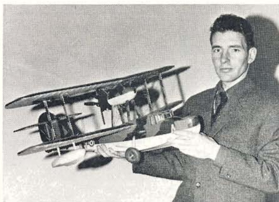
William Moesli's scale "Walrus" amphibian from A.P.S. plan was one of the entries in the last Model Engineer Exhibition. The model weighs 1½ lb. and is powered by a Cox Golden Bee.
