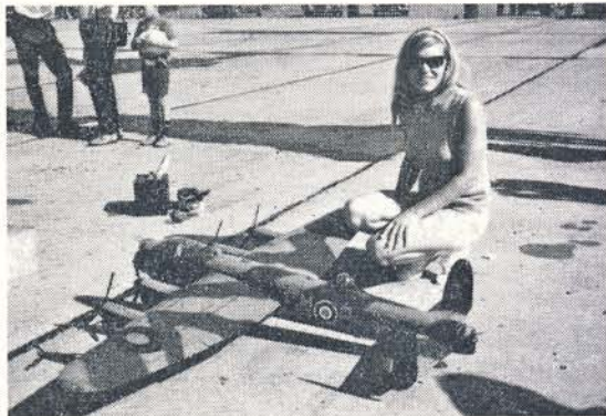
Judy Keith guards hubbie Keith's 16 lb. control line scale winning Avro Lancaster Mk.I. Feature opening bomb bay doors, flaps, moving turrets and lights. Retracting gear now fixed. Powered by four Super Tigre .23 engines.
