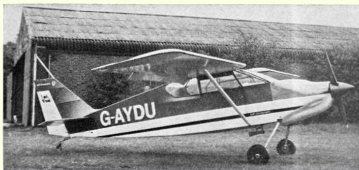
Above top, is a very early 'Tailwind', photographed in California before the minimum size of registration letters was introduced (just visible on rudder)! Beneath that is another view of the aircraft in its early stage - identified by the deeper cowl shape, lack of leg fairings and the external venturi tube. Smart colour scheme of metallic bronze and white aids appearance considerably. Below are details of the simple hydraulic braking system. Wheel spats are now under development.
