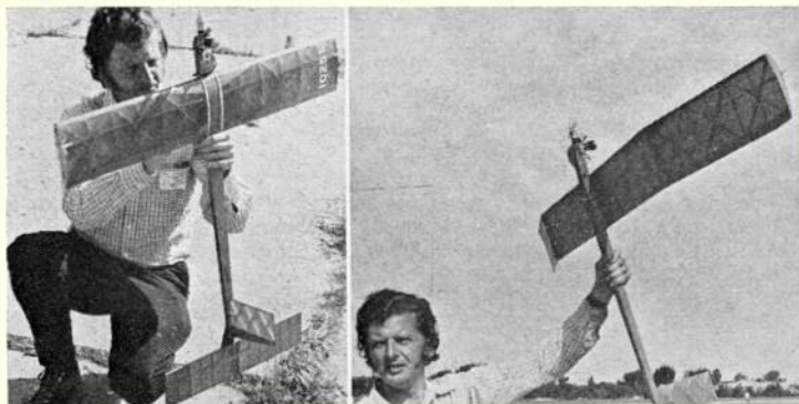
Jack McGillivray demonstrated his wing-folding Class A model. Glides like a well-tempered Nordic, engineering superb. Had trouble sorting out the climb 'pattern'. (A vertical straight line is a pattern?)
