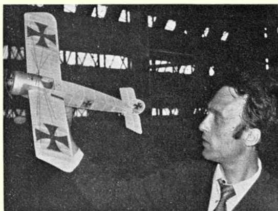
Terry Manley won the Indoor meeting with his Fokker E3 – an ideal subject for this class with its large wing, simple construction and low all-up weight. Small tailplane was its only drawback, making it tricky to trim.
