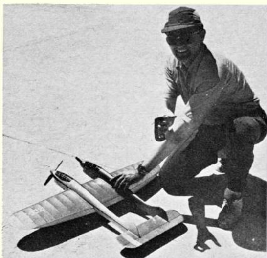
Above and below left. The perfect answer for single-handed flyers? Lines in this case are wrapped around the pulley shown below, so that the pilot starts his engine, then merely picks up his handle and releases the model, which rotates around the pulley until the lines are fully extended, and then the take-off is made in the normal way! Simple, and it works every time for its inventor, Frenchman François Couprie.
