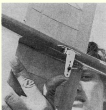
A trio of tow-hook ideas! At left, a 4-way steel tow mechanism by Ekhtenkov, although not used on his winning model. Above, Branco Leskosek's folding offset hook used for circular towing. At right, Lepps 4-way tow-hook is made from brass. Both Russian hooks obviously easily detachable.
