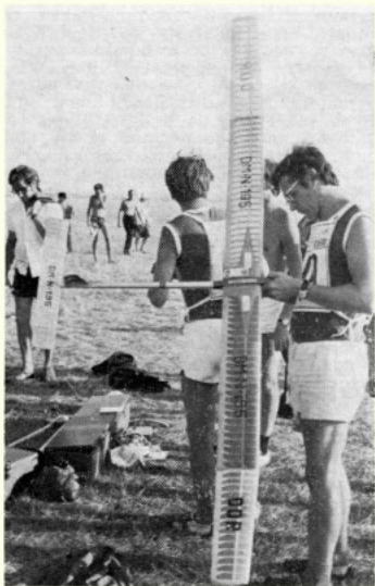
At left, East Germany Matthias Hirschel reached the massive fly-off at the Wiener Neustadt champs with this straightforward design with well-gusseted ribs, but placed no higher than an eventual 33rd. At right, Antonin Simerda of Czechoslovakia follows current trends with his high aspect ratio Wakefield with machined aluminium motor tube and forward fin.
