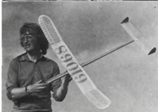
At top is Colin Hickmott (York) who was placed 4th in Open Power at the Leeds Rally with his Fox 15 powered model. Above is Steve Marriot with his Coupe d'Hiver model which features an octagonal balsa fuselage and is fitted with an Elmic D/T timer to operate the propeller start delay.
