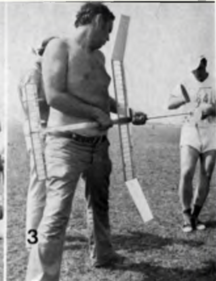
Wakefields all. 1. Albrecht Oschatz with Joakim Loffler behind (both previous World Champions) wait for signs of lift. 2. Jon Davis (and Sarah) - used his older 'Groovy Tuna' having damaged his new model earlier in practice. Preferring to wind with prop attached (protected by a metal disc) Jurov of USSR (3) uses transparent Melinax covering. 4. These Noel Coward cigarette holders are ideal for lighting D/T's! Actually, it's the well equipped Swiss team - note the yoke winder. 5. Mike Thomas (Canada) with Brian Egglestone on thermistor, was surprisingly the only one using delayed prop release. 6. 1971 World Champion Josef Klima came close to another chance of the title. 7. Peter Rasmussen of Denmark is left handed, so he carves his props backwards and trims left-left. 8. Smiles all round for the North Koreans - not surprising, Kim In Sul placed 4th individual. 9. A great performance from Australia's Alan Edwards - he narrowly missed the fly-off using his own instinct rather than resort to 'piggy backing'.
