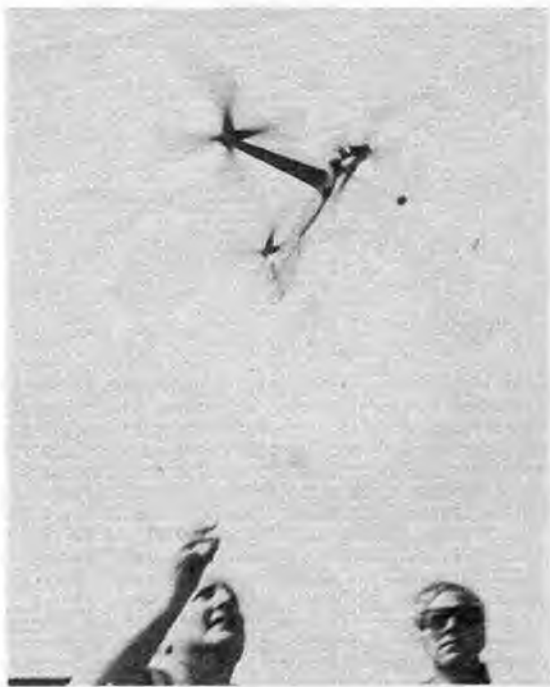
Airborne —and not a wing in sight! Tri-gyro makes a very different profile in the sky with its three rotors spinning wildly. Never throw the model—just let the blades build up to speed whilst walking forward before launch.
