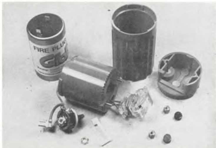
The Glo-Bee "Fire-Plug", the complete 'glowplug power-source' - built in rheostat enables current to be varied to suit all types of plug. Although Fusite Glo-Bee glow-plugs are imported by both Irvine Engines and Ripmax Ltd., neither concern at present have plans to import the accessories illustrated on these pages. Further details may be obtained from Fusite Division, Emerson Electric Co., 6000 Fernview Avenue, Cincinnati, Ohio 45212, U.S.A.
