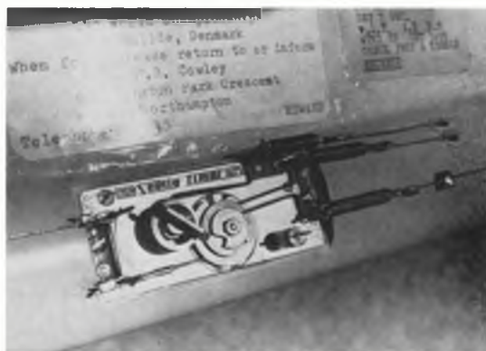
Close up of timer reveals (front) flood-off and brake lines, and (rear) dethermaliser, rudder and variable incidence lines. Note use of 'pre-flight' check list, pasted onto model next to (essential) address label.
