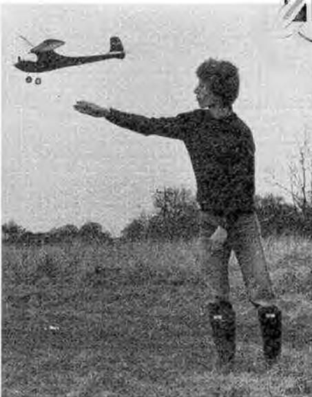
Above left: always get an assistant to restrain the model when starting the engine, leaving one hand free to adjust needle valve or compression, and prevent premature take offs! Above: test gliding is always the first stage before attempting powered flights. Look out for undesirable stalling or diving and watch for direction of glide turn.
