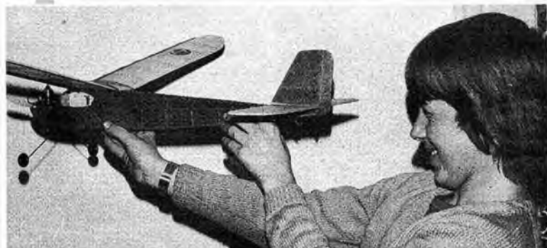
Check assembled model for unwanted wing or tail tilt, or for excessive warps and correct, using shims of packing or dewarping with steam before attempting to fly the model.
