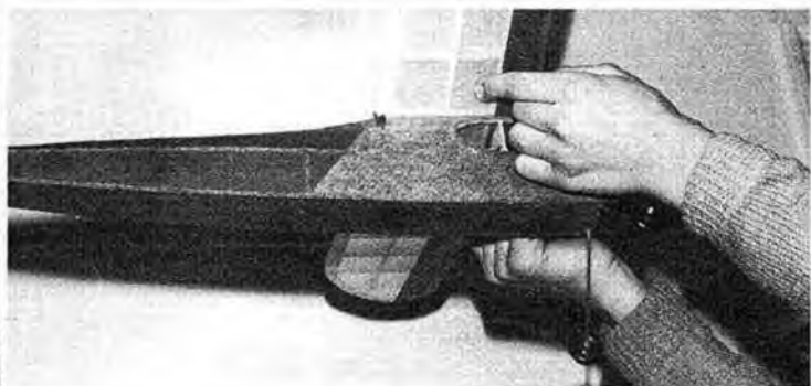
Support the assembled model under the wings to ensure the model balances exactly at the position indicated on the plan. Add weight at nose or tail to correct.
