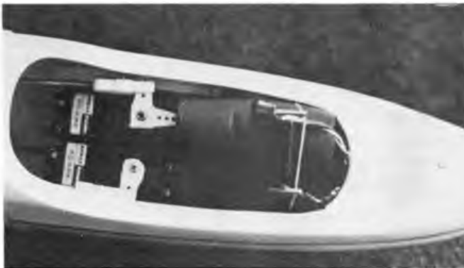
Neat exit for the elevator push pull rod. Note the film covering the elevator hinge line, bolt on elevator horn and rubber bands holding tailplane. Below, servos and radio installation. I held the receiver on-off switch to receiver rubber packing with a band. Alternatively a strip of A.B.S. plastic is supplied in the kit to make a bracket for the switch.
