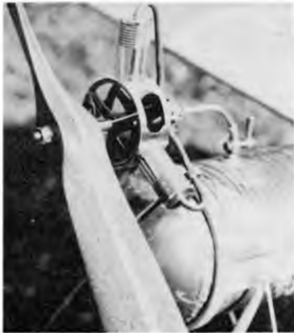
Left, close up of the F. J. Camm designed 3 cylinder compressed air engine made by Tony Turner. A pressure of 60 psi in the container causes the 18 inch diameter laminated Pavely tape propeller to dissolve into a disc of spinning light. Tony Turner's compressed air powered model about to ROG at Old Warden. This machine with kingpost bracing, spoked wheels and "toothpick" skid is a free lance design based on the practice of D. A. Pavely, who was the leading exponent on compressed air in this country before the war.
