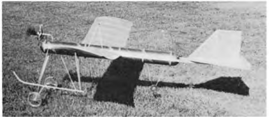
Left, close up of the F. J. Camm designed 3 cylinder compressed air engine made by Tony Turner. A pressure of 60 psi in the container causes the 18 inch diameter laminated Pavely tape propeller to dissolve into a disc of spinning light. Tony Turner's compressed air powered model about to ROG at Old Warden. This machine with kingpost bracing, spoked wheels and "toothpick" skid is a free lance design based on the practice of D. A. Pavely, who was the leading exponent on compressed air in this country before the war.
