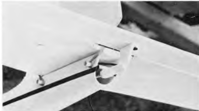
Neat exit for the elevator push pull rod. Note the film covering the elevator hinge line, bolt on elevator horn and rubber bands holding tailplane. Below, servos and radio installation. I held the receiver on-off switch to receiver rubber packing with a band. Alternatively a strip of A.B.S. plastic is supplied in the kit to make a bracket for the switch.
